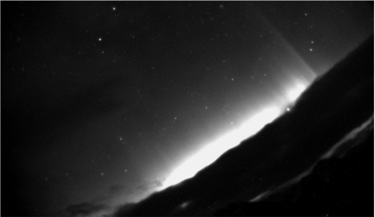
Fig. 6. Aurora image taken with the demokit of the ONYX detector during the Ny-Ålesund Nov 2017 campaign. The exposure time is 0.82 s, the analog gain is \times 6 . The instrument was inclined at about 45^\circ . The aurora was faint, barely visible with naked eyes.
