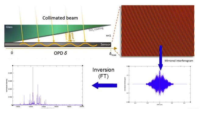
Fig. 1. Schematic representation of the SPOC principle.
