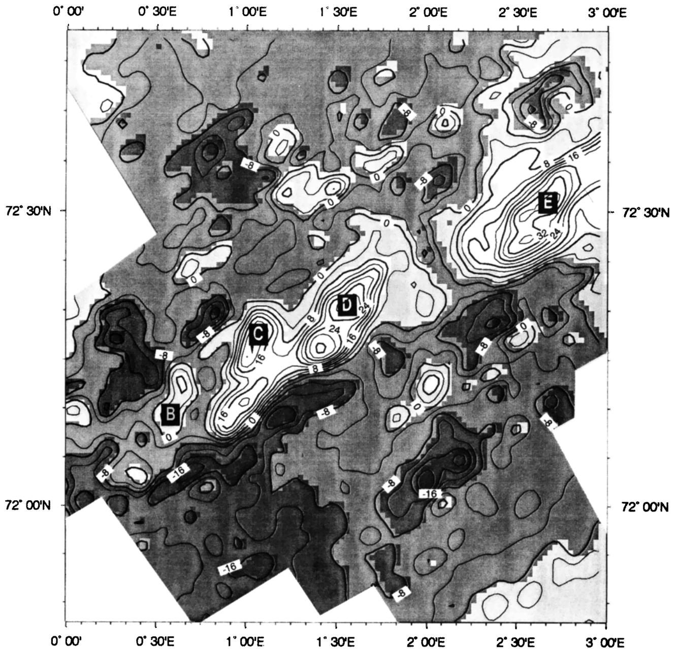
Fig. 6. Distribution of source rock magnetization (A/m). Inversion of the magnetic anomalies in presence of topography was performed using the *Parker and Huestis* [1974] method, assuming a uniform, 500 m thick, magnetized layer parallel to the seafloor. The amount of annihilator that was added to the solution was found by balancing the positive and negative magnetization on each side of the polarity boundary. See Figure 3 legend.
