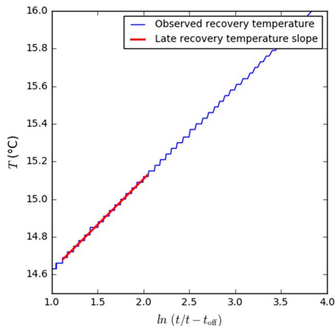
**Figure 8.** Observed temperatures during the recovery period for the submersible sensor located at 53.6 m depth for the test with a continuous heating cable.
