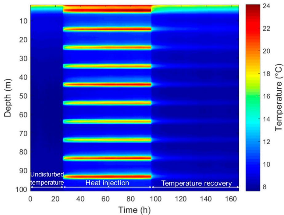
**Figure 4.** Temperature evolution during the three steps of the TRT in Quebec City with heating cable sections.
