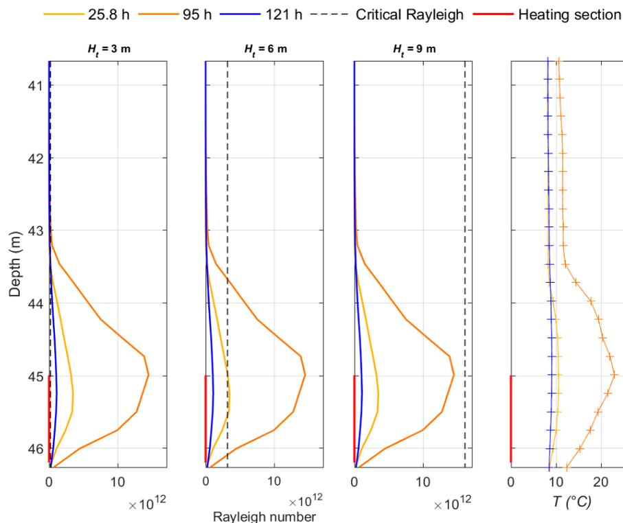
**Figure 11.** Verification of the Rayleigh number stability criterion considering different critical lengths  $H_t$  to calculate the critical Rayleigh number (dashed lines) for the test with heating cable sections.
