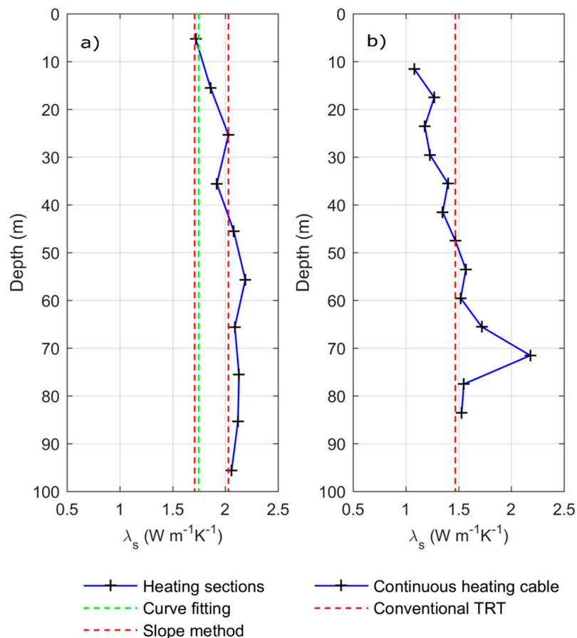
**Figure 9.** Point subsurface thermal conductivity (crosses) obtained with the (a) heating cable sections in Québec City and (b) the continuous heating cable in Orléans. The results are compared to the bulk values provided by the conventional TRT with water circulation (green and red dashed lines).
