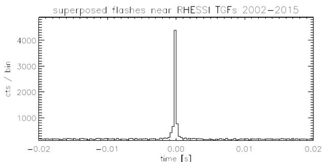
**Figure 3.** A total of 383 superposed Reuven Ramaty High Energy Solar Spectroscopic Imager (RHESSI) datastrings corresponding to World Wide Lightning Location Network detections occurring within 1 ms of an identified terrestrial gamma ray flash (TGF) in the Gjesteland et al. (2012) catalog, and binned with 250  $\mu$ s.
