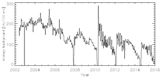
**Figure 2.** The average number of counts in the collected Reuven Ramaty High Energy Solar Spectroscopic Imager datastrings, binned at 10-day intervals. We see the average count rate decreasing until an anneal is performed (when there are no data), temporarily increasing the sensitivity. The missing data in late 2002 are not due to an anneal, but missing World Wide Lightning Location Network data.
