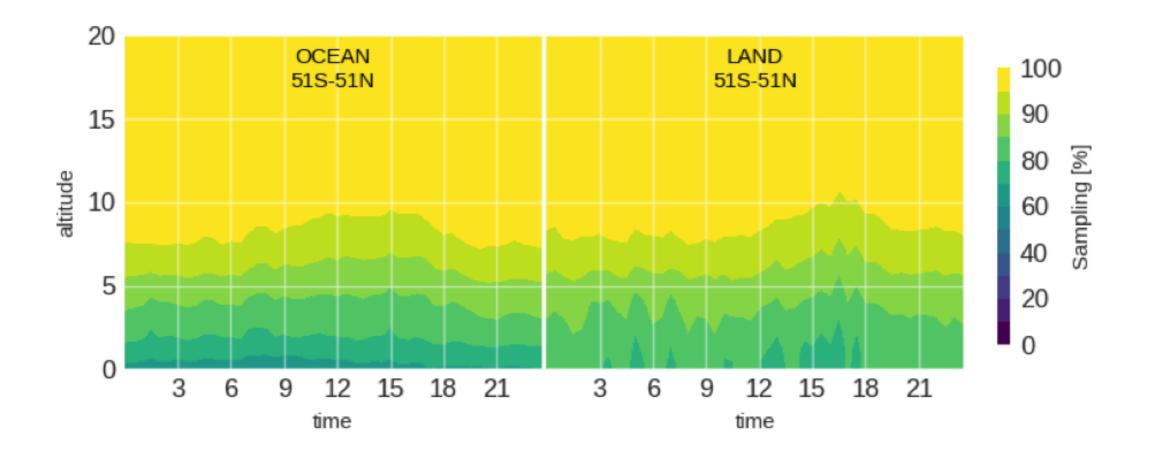
Even though some profiles get fully attenuated by atmospheric components, sampling is better than 80% at most altitudes, and ~100% above 7km except late in the afternoon
