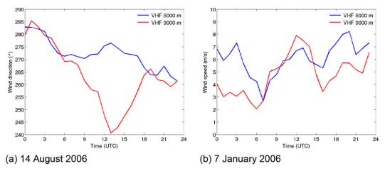
FIG. 6. Typical diurnal evolution of (a) wind direction (14 Aug 2006) or (b) wind speed (7 Jan 2006) as observed from the VHF radar at 3000 and 5000 m MSL.
