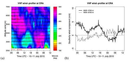
FIG. 3. (a) Horizontal wind vectors retrieved from the VHF wind-profiler at CRA, from 0000 UTC 10 Jul 2010 to 1200 UTC 11 Jul 2010. The color code represents the wind direction. The length scale of the vectors is given in red in the bottom-left corner. (b) Southerly component of the VHF wind vertically averaged between 2675 and 3750 m MSL (thick curve) and between 4500 and 6750 m (thin curve).
