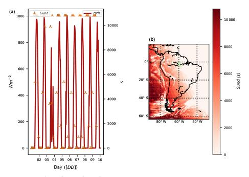
**Figure 2.** Temporal evolution at  $62^{\circ}4'38.00''$  S,  $4^{\circ}58'55.51''$  W (a) of shortwave downward radiation (rsds, red line, left *y* axis) and sunshine duration for a 3-hourly 9freq (sund, stars, right *y* axis). (b) Sunshine length map on 9 December 2012 at 15:00 UTC. X denotes the position of the temporal evolution.
