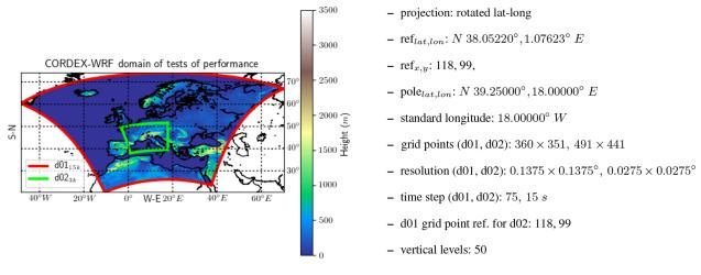
Figure 17. Two-nested domain WRF3.8.1 configuration in which different performance tests were carried out.
