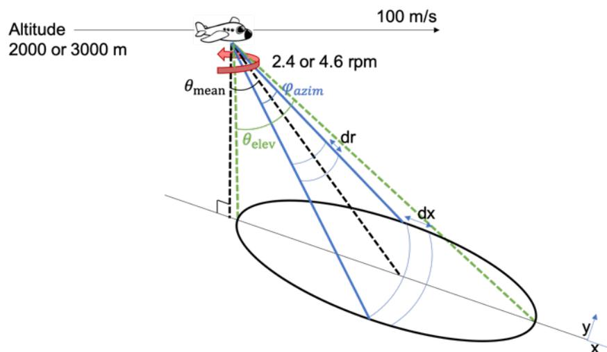
**Figure 1.** Schematic view of the KuROS radar. Here, only the LI (low incidence) antenna is indicated as this paper focusses on data acquired only with this antenna.  $\theta_{\text{mean}}$ ,  $\theta_{\text{elev}}$ ,  $\varphi_{\text{azim}}$  stand for the mean elevation angle, the antenna one-way 3 dB
