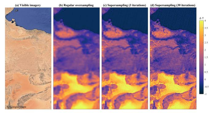
**Figure 2.** Illustration of the IBP superresolution technique on IASI observations of a BTD sensitive to surface quartz. All cloud-free observations of IASI for the period 2007–2018 were used for the averages. Panel (a) shows the corresponding visible imagery from Google Maps.
