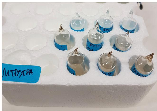
**Fig. 3.** The MTBSTFA flame-sealed ampoules in their styrofoam holder. Blanks (top row), 150 krad (middle row) and 300 krad (bottom row). A darkening of the borosilicate ampoule was observed after irradiation.
