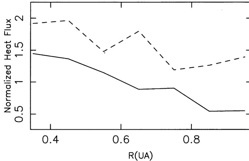
FIG. 2.—Normalized heat flux from 0.3 to 1 AU, obtained from the values of the macroscopic parameters determined by Marsch (1982) and Marsch et al. (1982) from the *Helios* measurements. The solid line corresponds to the slow winds ( $300\text{--}400\text{ km s}^{-1}$ ) and the dashed line to the fast winds ( $600\text{--}700\text{ km s}^{-1}$ ).
