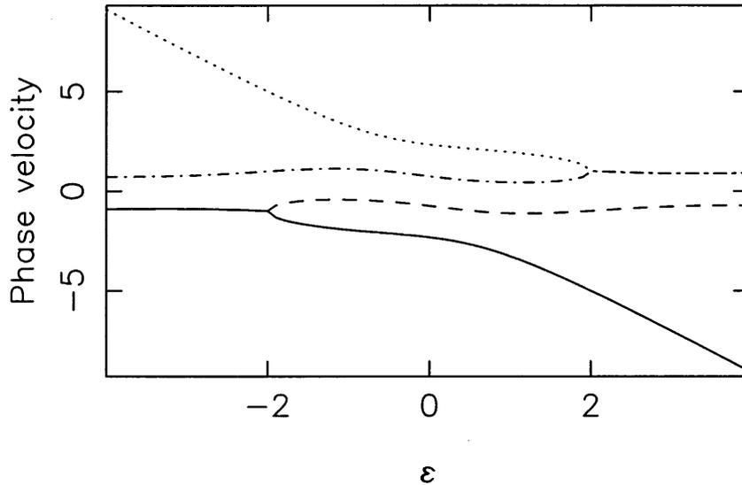
FIG. 1.—Dependence of the four phase velocities solution of the characteristic polynomial (see eq. [23]) as a function of the  $\epsilon$  parameter. From  $|\epsilon| > 2$ , we have represented the real part of the complex solution.
