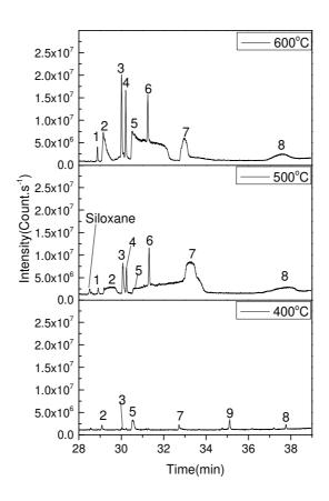
Figure 4: Chromatograms of guanine (11 nmol) thermochemolysis in TMAH at 600 °C, 500 °C, and 400 °C. (1: caffeine; 2: dimethyl-guanine; 3 and 5: trimethylguanine; 4, 6, 7, 8: tetramethylguanine; 9: trimethylguanine).
