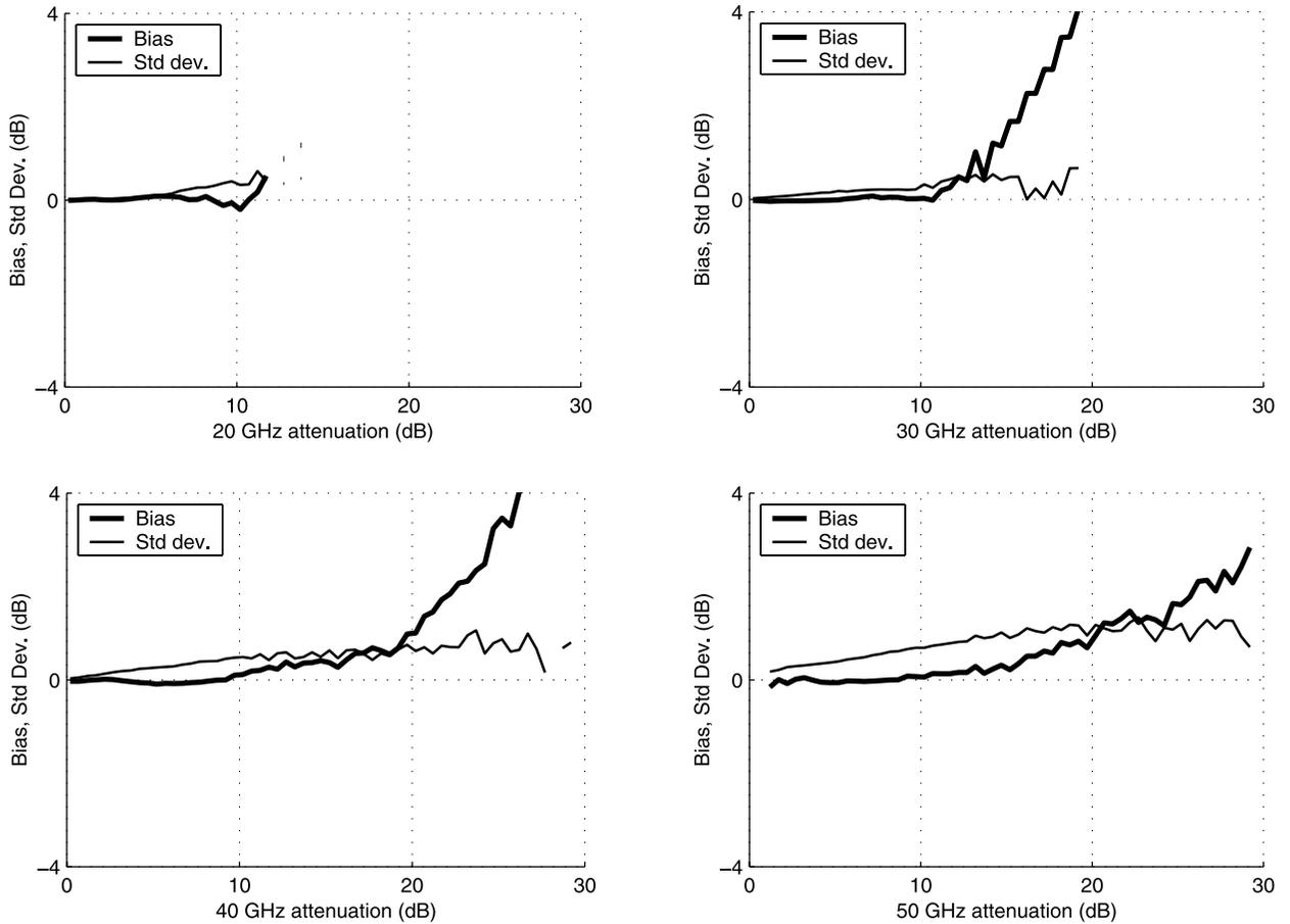
**Figure 4.** Generalization error of the NN attenuation model at 20, 30, 40 and 50 GHz obtained on simulated data. The thick line corresponds to the error bias, and the thin line corresponds to the standard deviation error as a function of attenuation.
