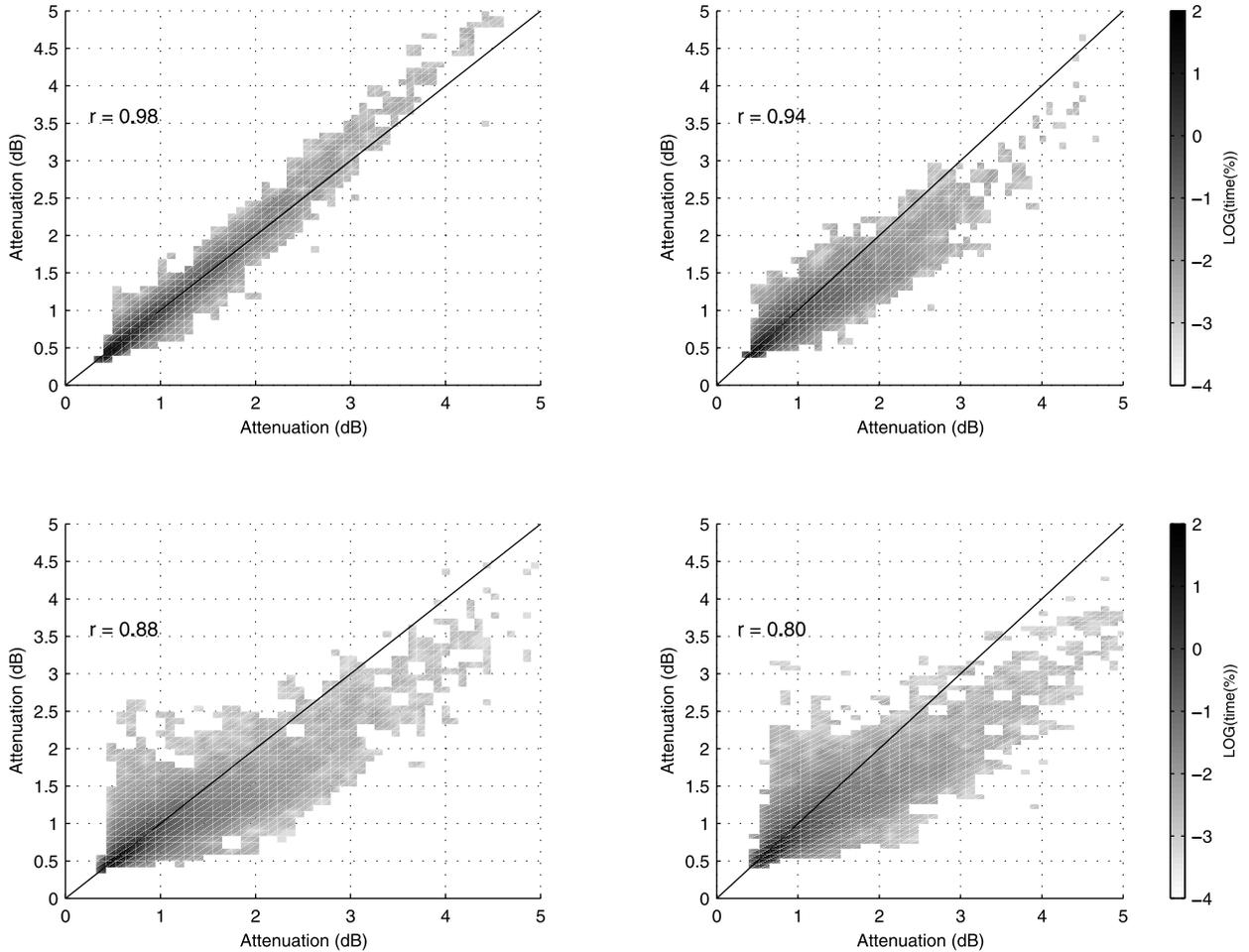
**Figure 10.** Joint statistics between atmospheric attenuation observed for four different pairs of angles  $(\theta_1, -\theta_1)$  at 40 GHz. The corresponding correlation coefficients are given. Angle pairs, from left to right, and top to bottom:  $5^\circ, 18^\circ, 23^\circ, 41^\circ$ . See color version of this figure at back of this issue.
