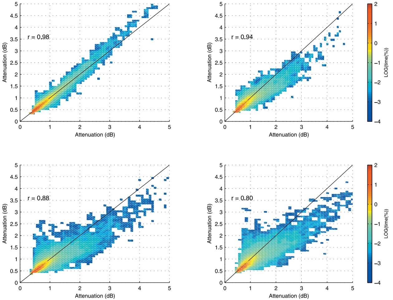
**Figure 10.** Joint statistics between atmospheric attenuation observed for four different pairs of angles  $(\theta_1, -\theta_1)$  at 40 GHz. The corresponding correlation coefficients are given. Angle pairs, from left to right, and top to bottom:  $5^\circ$ ,  $18^\circ$ ,  $23^\circ$ ,  $41^\circ$ .
