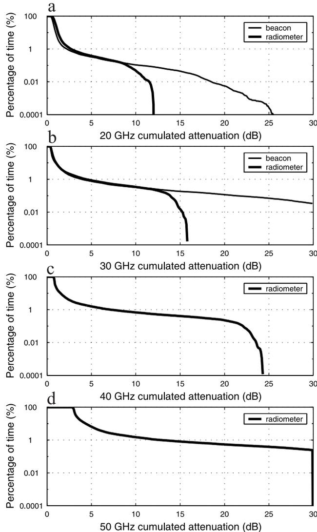
**Figure 7.** Exceedance time percentages of attenuation estimated by means of the Olympus beacons (thin) or deduced from radiometer measurements by means of the NN model (thick). Frequencies of (a) 20, (b) 30, (c) 40, and (d) 50 GHz are shown.
