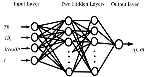
**Figure 3.** Architecture of the neural network developed. Four inputs: a pair of brightness temperatures  $TB$  at two different frequencies  $f_1$  and  $f_2$ , the cosecant of zenith angle  $\theta$  and the frequency ( $f$ ). One output: the atmospheric transmissivity at frequency  $f$  and zenith angle  $\theta$ .
