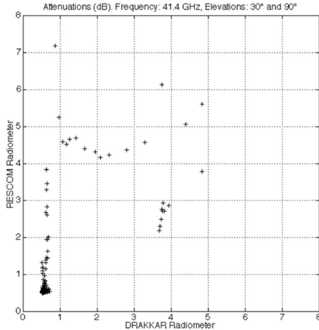
**Figure 9.** Evolution of the 40 GHz attenuation at two pointing directions: The zenith attenuation is shown on the x axis, and the attenuation measured for a 60° zenith angle towards the west is shown on the y axis.
