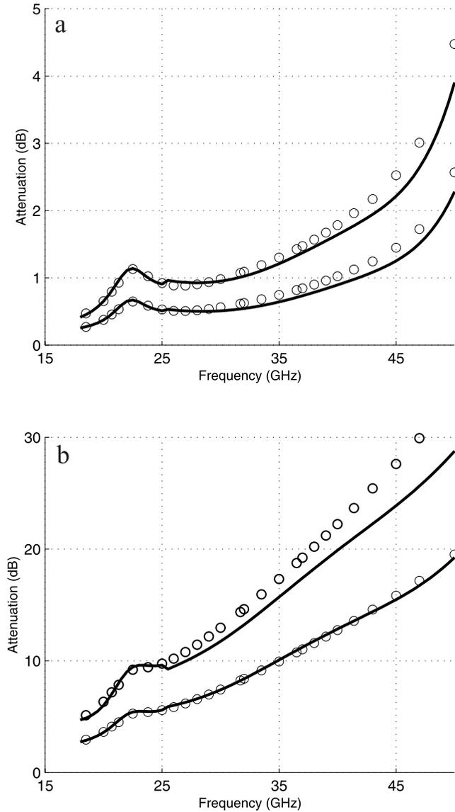
**Figure 5.** Attenuation versus frequency obtained for two particular atmospheric profiles corresponding to (a) low and (b) high attenuation situations, respectively. In each figure part the two curves correspond to two zenith angles: (bottom)  $0^\circ$  and (top)  $60^\circ$ .
