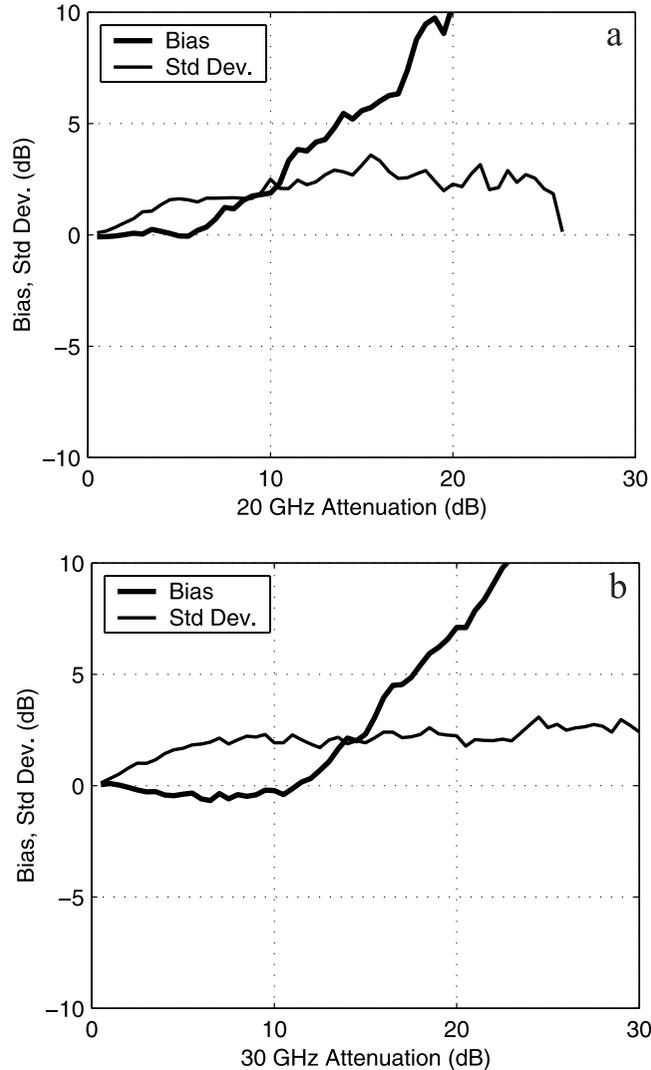
**Figure 6.** Generalization error of the NN attenuation model at (a) 20 and (b) 30 GHz obtained on actual data measured during the Olympus experiment. The thick line corresponds to the error bias, and the thin line corresponds to standard deviation error as a function of attenuation.
