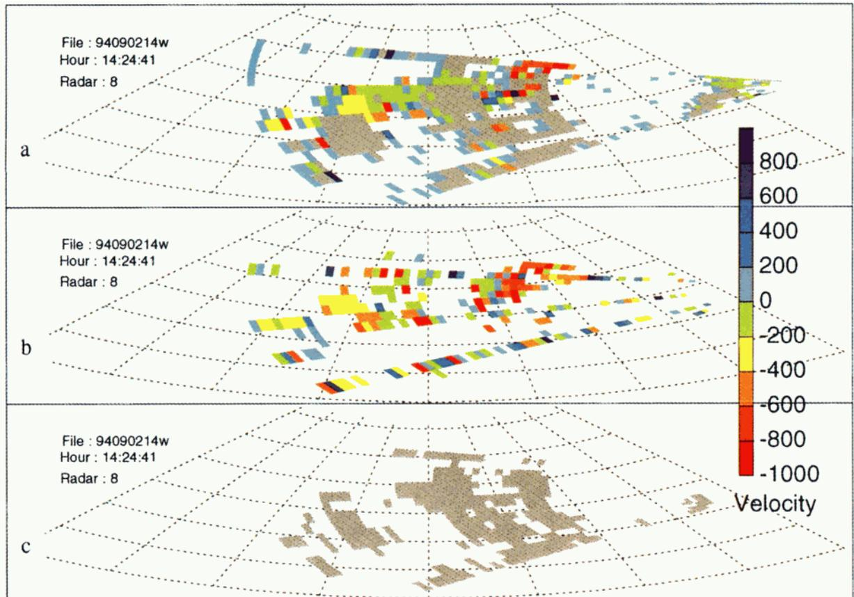
**Plate 1.** Radial velocity maps obtained with the Stokkseyri SuperDARN radar, showing (a) the velocity obtained with the standard analysis; (b) the ionospheric echoes detected by MUSIC; and (c) the ground scatter echoes detected by MUSIC. The coordinates are geographic latitude and longitude.
