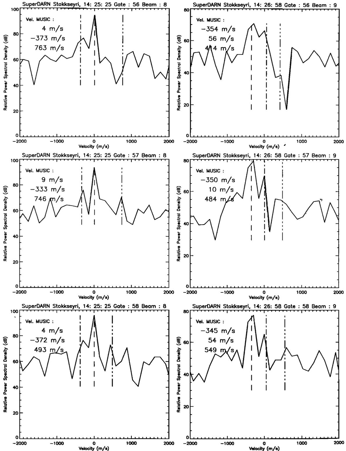
**Figure 7.** Comparison between the results of MUSIC and a fast Fourier transform (FFT) analysis of the ACF in six adjoining cells. The multiple sources detected by MUSIC in the different cells are mutually consistent.
