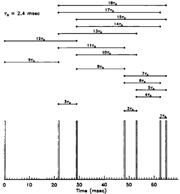
**Figure 1.** Example of a seven-lag multipulse scheme used by the Super Dual Auroral Radar Network (SuperDARN) radars. This sequence allows determining 17 points of the autocorrelation (ACF) function of the backscattered signal.
