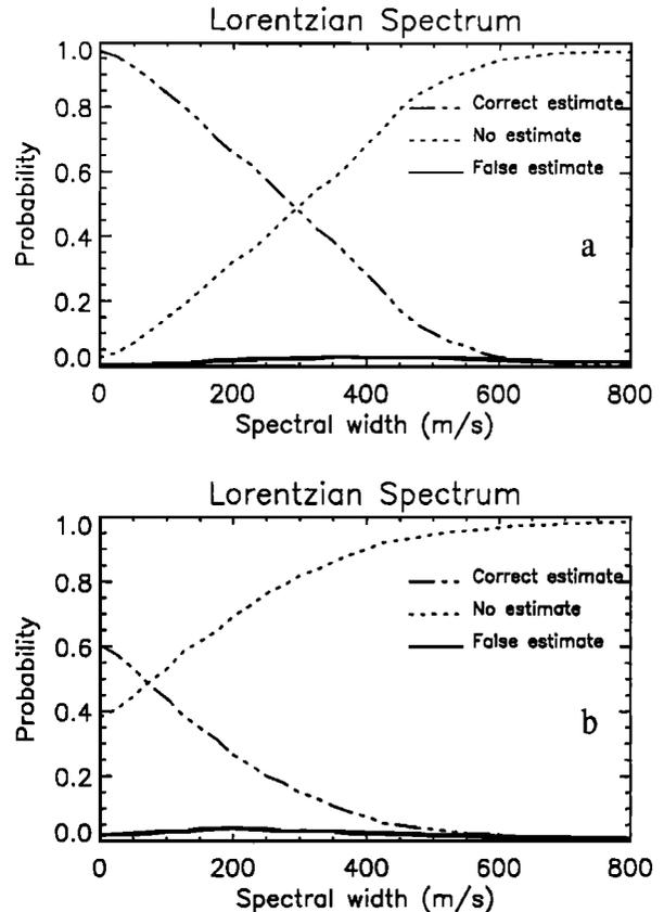
**Figure 6.** Statistical results of the MUSIC analysis when two sources (ionospheric and ground) are present in the signal. The probabilities of different results (correct, false, or no velocity determination) for a Lorentzian ionospheric source are presented. (a) The source separation is larger than the resolution of the Fourier analysis. (b) The source separation is smaller than the resolution of the Fourier analysis.
