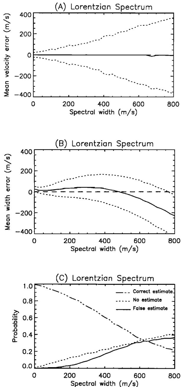
**Figure 4.** Statistical results of the simulation of the analysis of the SuperDARN ACFs with the multiple signal classification (MUSIC) algorithm. (a) Mean error (solid line) and variance (dotted line) in the velocity determination. (b) Mean error (solid line) and variance (dotted line) in the spectral width determination. (c) Probabilities of different results of the MUSIC analysis (correct, false, or no velocity determination). The ACF comprises one single source with a Lorentzian spectrum.
