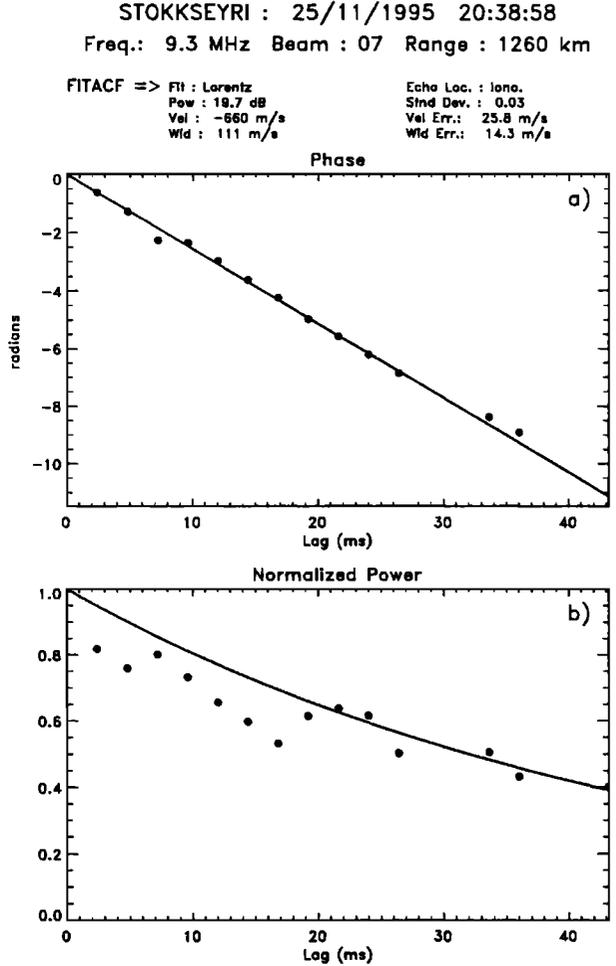
**Figure 2.** Illustration of the "standard" analysis of the SuperDARN ACFs. (a) The Doppler frequency is determined by a linear least squares fit of the phase of the ACF. (b) The spectral width is deduced from the fit of the power to a Gaussian or a Lorentzian spectrum.
