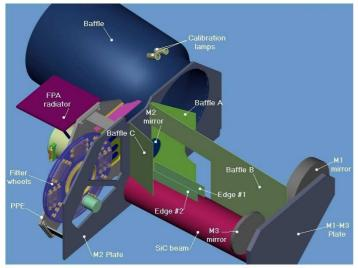
Fig. 3. Two schematic views of the OSIRIS Narrow Angle Camera.
