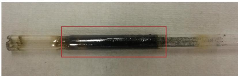
Figure 8. Picture of the dark residues deposited in the gas chromatograph-mass spectrometer liner after the exposure to 600 °C of 50 mg of Tenax ® GR contained in the liner.
