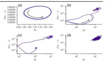
FIG. 4. Phase trajectory of the flow and core temperature for systems at Pr = 0.03,  $Ek = 3 \times 10^{-6}$ , and [(a),(c)]  $Ra = 1.03Ra_{crit}$  and [(b),(d)]  $Ra = 1.1Ra_{crit}$ . The top row [(a),(b)] shows runs initialized from a weak branch state; the bottom row [(c),(d)] shows runs initialized from a strong branch state. The lines get darker as the system evolves. The arrows in (a) and (b) indicate the direction of time.
