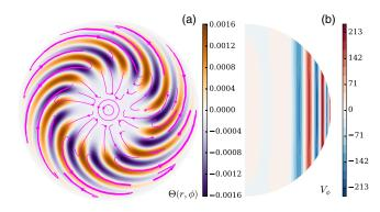
FIG. 2. Cross sections of the weak branch system at  $Ek = 10^{-6}$ , Pr = 0.01,  $Ra = 5.53 \times 10^7 = 1.01 Ra_{crit}$  showing (a) the temperature profile in the equatorial plane. Streamlines of the flow in the plane are plotted over the temperature profile in pink. (b) Meridional slices of the azimuthal velocity.
