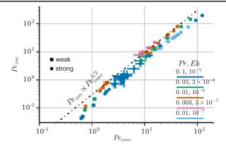
FIG. 5. The averaged zonal velocity  $Pe_{zon}$  of the flows as a function of the averaged convective velocity  $Pe_{conv}$ . Ek and Pr are indicated by color. The shape of the markers indicates the branch the averages were taken over. The error bars represent fluctuation levels.
