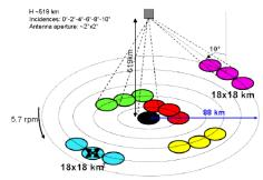
Fig. 1 SWIM beam rotation and incidence angles.
