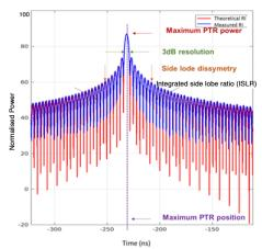
Fig. 2 Point Target Response (PTR). Blue line: measured, red line: theoretical sinus cardinal function.
