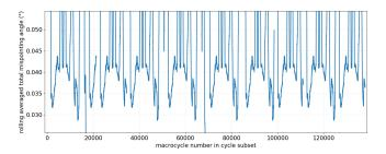
Fig. 3 Rolling average of the total mispointing angles estimated in the level 1A processing over several orbits of 1.5h each, with respect to macrocycle number in the selected subset. Values are averaged over 500 macrocycles. The oscillations show the impact of the reference ellipsoid.
