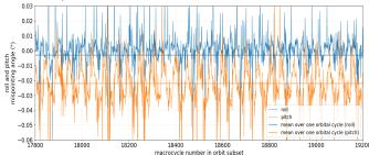
Fig. 4 Zoom of roll (blue curve) and pitch (orange curve) mispointing angles estimated in the level 1A processing over about 5 minutes. The thick blue and orange horizontal lines show the mean roll and pitch angles, respectively, averaged over one cycle of data (13 days).
