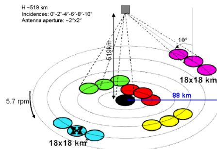
Figure 1 SWIM beam rotation and incidence angles
