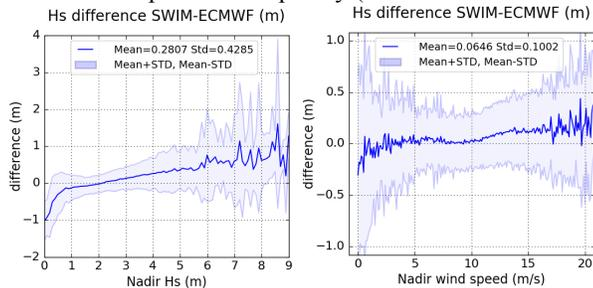
Figure 6: Difference between SWIM and ECMWF significant wave height. Left: as a function of significant wave height; right: as a function of wind speed. Blue/light blue: mean/one std envelope..
