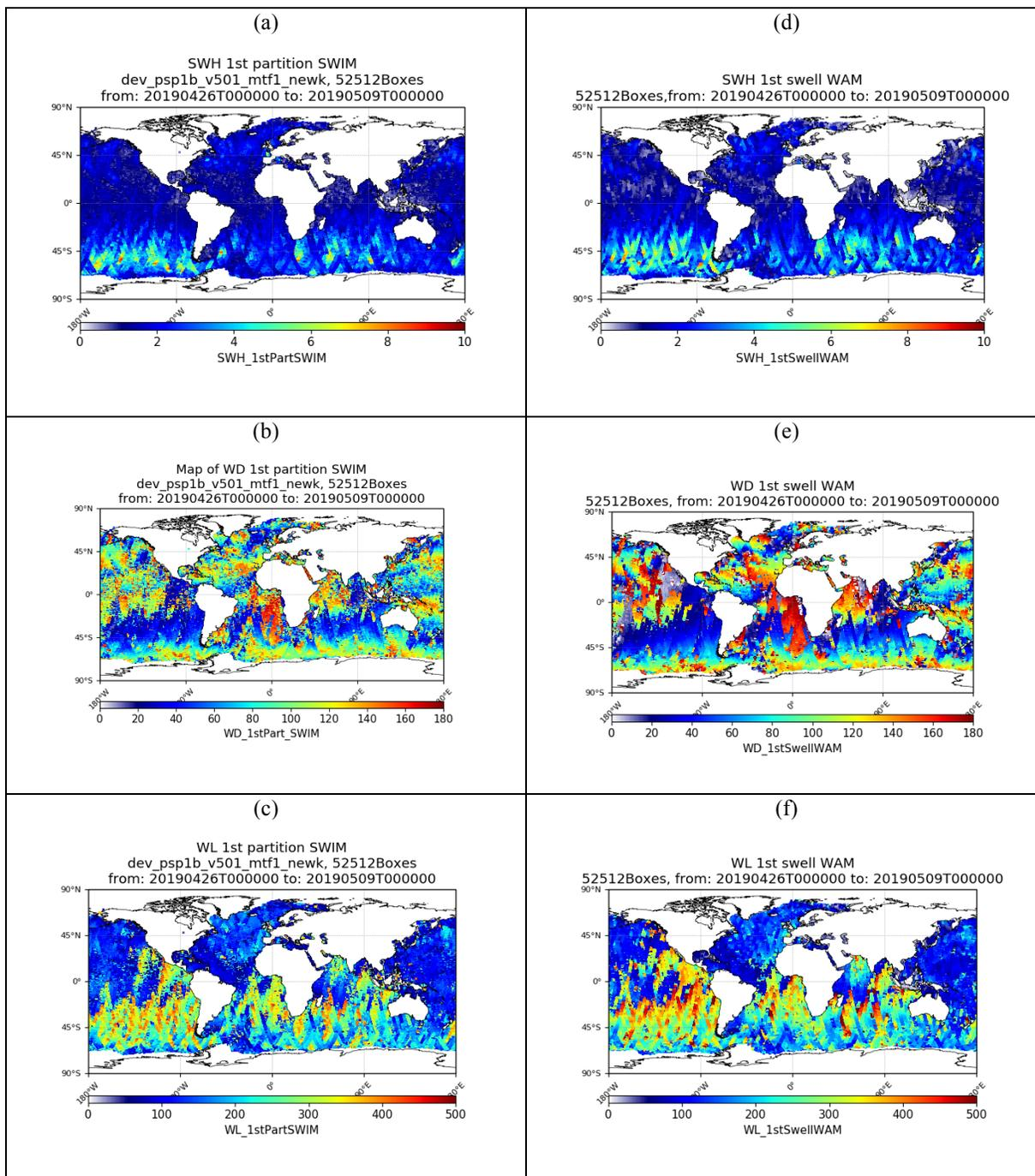
Figure 20 : Maps of SWIM (a, b, c) and MFWAM (d, e, f) parameters for a period of about 13 days starting on April 26<sup>th</sup> 2019 02 :00. a and d: wave height of the first partition; b and e: direction of the first partition (for MFWAM the directions have been folded in the [0-180°] interval to be compared with the SWIM data); c and f: wavelength of the first partition. The SWIM results are shown for the 10° incidence beam. See text for details.
