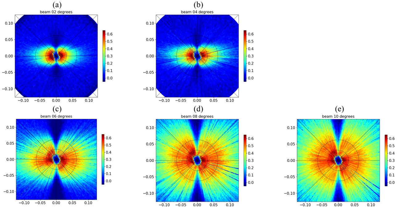
Figure 13: Polar plots of the correlation coefficient between SWIM fluctuation spectra and WW3 collocated wave slope spectra for the data set from April, 25<sup>th</sup> to April, 30<sup>th</sup>, 2019. Horizontal and vertical axes refer to the wave number of the waves in two orthogonal directions, with the vertical axis aligned with the satellite along-track direction. Panels (a, b, c, d, e): for SWIM beams 2°, 4°, 6°, 8°, 10°, respectively.
