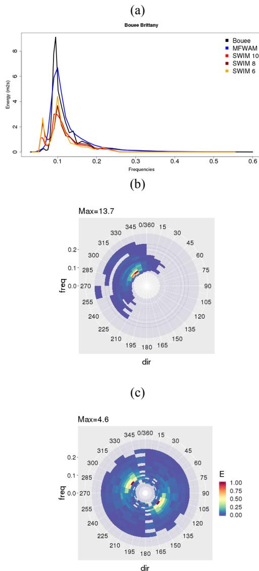
Figure 21(a) Omni-direction spectra ( $m^2/s$ ) from the Brittany buoy (47°33’0” N 8°28’12” W), MFWAM and SWIM (3 beams with the red, brown and yellow curve as indicated in the insert) on August 19<sup>th</sup> 2019 18:00 UTC. (b, c) directional spectrum from (b) the buoy, (c) SWIM beam 10°. In (b, c), the color scale is relative to the maximum of energy of each plot.
