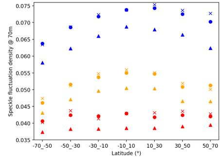
Figure 16: Speckle noise spectral level at  $k = 0.09$  rad/m (wavelength of  $\sim 70$  m), calculated from our empirical formulation, at the azimuth angle of maximum speckle level ( $\phi = \phi_0$ ). The results are plotted for the three SWIM beams in blue (6°), orange (8°), red (10°) and for three sea surface conditions (circle:  $H_s < 2m$  &  $U < 5m/s$ , cross:  $2m < H_s < 4m$  &  $5 < U < 9m/s$ , triangle:  $H_s < 2m$  &  $5 < U < 9m/s$ ).
