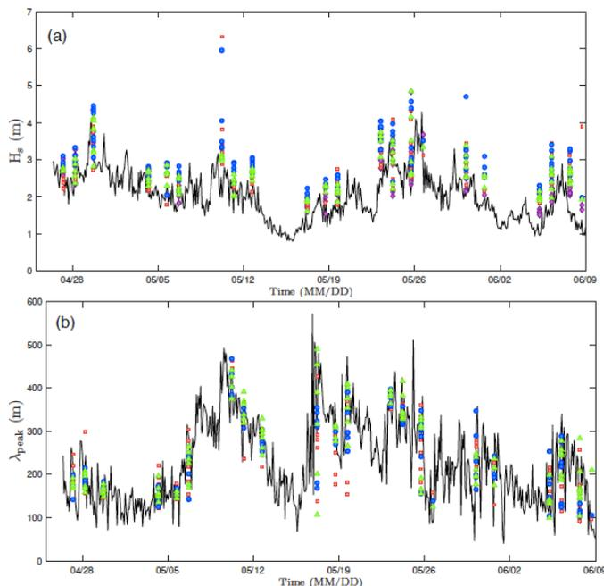
Figure 23: Time series of (a)  $H_s$  in m (b) peak wavelength in m from SWIM and from the OSSI probe in Moorea ( $-149.82^\circ\text{E}$ ,  $-17.61^\circ\text{N}$ ) between April 28<sup>th</sup> 2019 and June 9<sup>th</sup> 2019. The black curve indicates the in situ measurements. The CFOSAT nadir measurements are reported in magenta in panel a. The CFOSAT 6, 8 and  $10^\circ$  beams are reported in red, blue and green (panels a and b).
