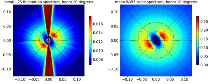
Figure 12: Mean fluctuation spectra for the period from April 25<sup>th</sup> to April 30<sup>th</sup> 2019 (left) compared to the mean wave slope spectrum obtained from collocated points of WW3 outputs (right). Horizontal and vertical axes refer to the wave number of the waves in two orthogonal directions, with the vertical axis aligned with the satellite along-track direction.
