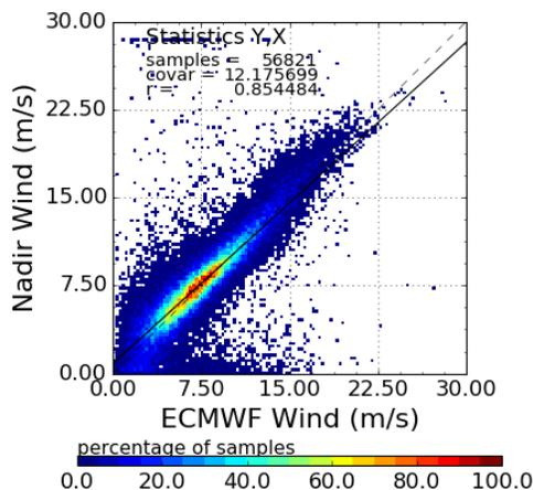
Figure 9: SWIM nadir wind speed compared to ECWMF wind speed for a 13-day period (9-21 September 2019)
