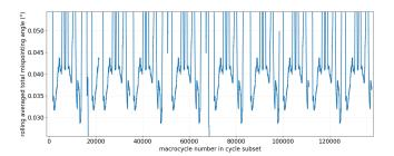
Figure 3: Rolling average of the total mispointing angles estimated in the level 1A processing over several orbits of 1.5h each, with respect to macrocycle number in the selected subset. Values are averaged over 500 macrocycles. The oscillations show the impact of the reference ellipsoid.
