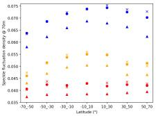
Figure 16: Speckle noise spectral level at k=0.09 rad/m (wavelength of  $\sim 70$  m), calculated from our empirical formulation, at the azimuth angle of maximum speckle level ( $\phi=\phi_0$ ). The results are plotted for the three SWIM beams in blue (6°), orange (8°), red (10°) and for three sea surface conditions (circle: Hs < 2m & U < 5m/s, cross: Hs < 2m & U < 5m/s, triangle: U < 5m/s.
