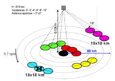
Figure 1 SWIM beam rotation and incidence angles
