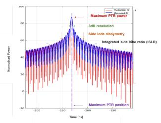
Figure 2: Point Target Response (PTR). Blue line: measured, red line: theoretical sinus cardinal function.
