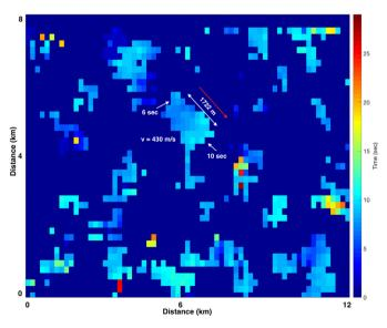
Fig. 4. Part of the image showing an example of detected perturbation. The example show a perturbation propagation at the sound speed with a 5 s period. The direction of propagation is manually deduced by following the color gradient and shown by the red arrow, consistent with waves originating from the northwestern.
