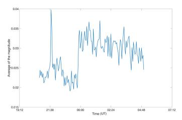
Fig. 9. Average of the magnitude of the pressure profile divided into 144 parts in the range [2–6] seconds.
