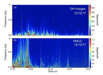
Fig. 8. (a): Wavelet transform of the OH radiance profile between 0,1 and 0,01 Hz for the entire night. (b): Wavelet transform of the pressure profile measured at ground with microsensors.
