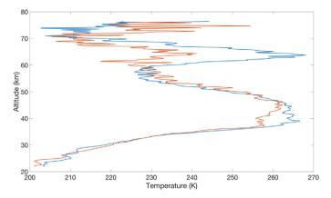
Fig. 6. Rayleigh lidar temperature profiles. The blue curve represents the average temperature for each altitude during the temperature inversion and the red curve is the average temperature after the inversion.
