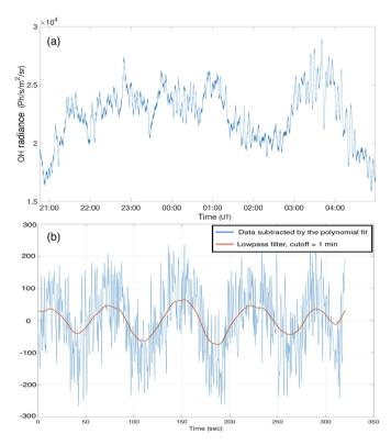
Fig. 3. (a): Temporal OH radiance profile of the 12–13 December at the OHP. (b): Portion of the OH radiance profile at the beginning of the night smoothed by applying a lowpass filter with a one minute cutoff period (red line). A dominant oscillation of  $\sim$ 75 s is noted.
