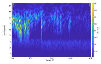
Fig. 1. Wavelet analysis of the pressure profile measured by the sensitive microbarometer during the night of the 12-13 December at OHP. The magnitude band centered on 0.25 Hz is visible at the bottom of the figure.
