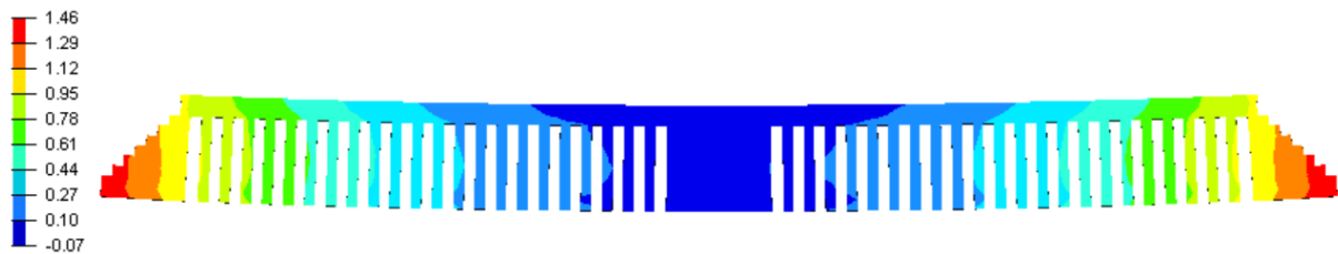
Figure 5: Displacement in Z direction with Accurate mode and constant Young's modulus E = 125 GPa.
