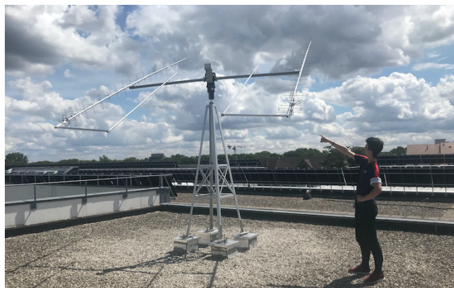
Figure 5. UVSQ/LATMOS UHF/VHF station (one of the stations of the INSPIRE network). LATMOS hosts students from UVSQ and Paris Saclay universities to provide hands-on experience (satellite manufacturing, antenna realization, etc.).
