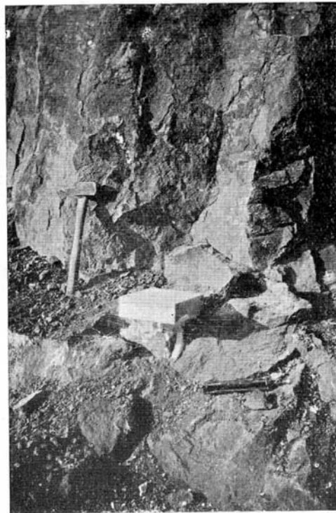
Figure 14. Method of orienting and collecting rock samples using a “plaster of Paris cap” (“chapeau de plâtre”) pioneered by E. Thellier [from Thellier , 1938, Figures 44 and 45].
