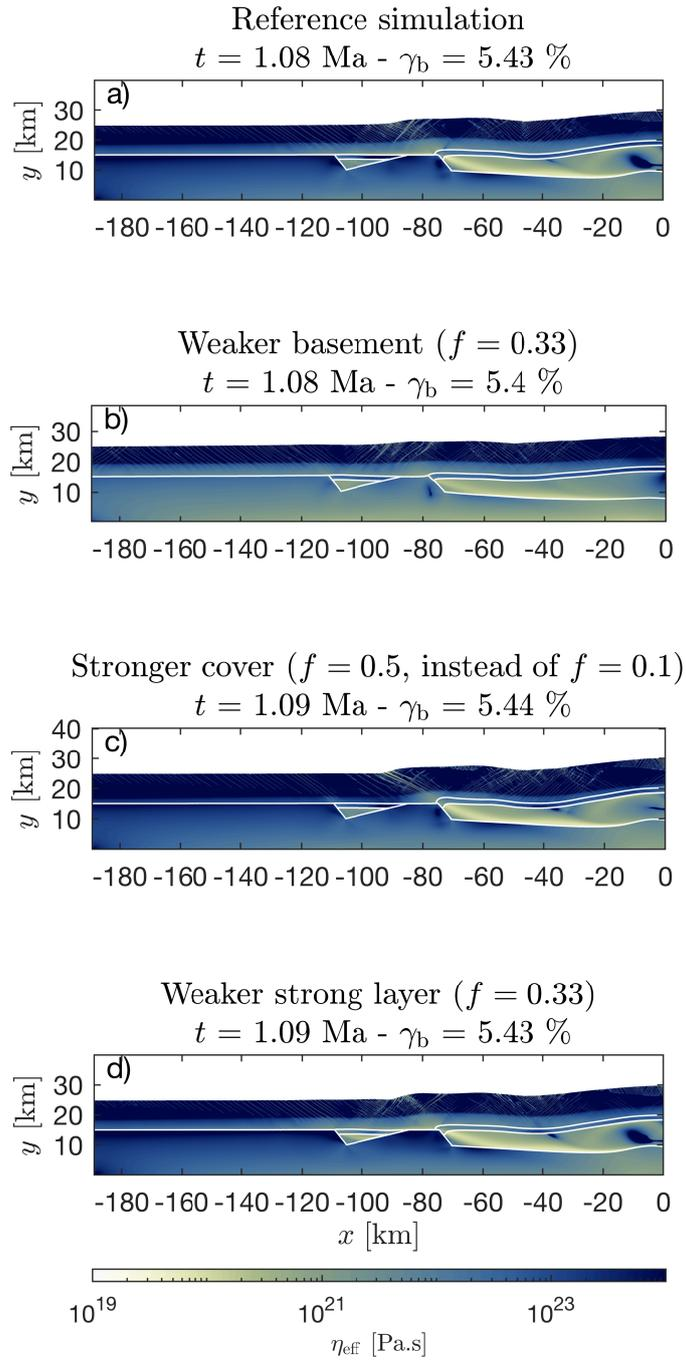
**Figure 7.** Effective viscosity for four simulations with different  $f$  factor for certain model units after a bulk shortening of ca. 5.4%. Below the brittle-ductile transition the effective viscosity (i.e. ratio of stress and visco-elastic strain rate) essentially equals the viscosity calculated from the dislocation creep flow law (eq. 1). Panel a) displays the reference simulation and panels b) to d) displays the three simulations shown in figure 6.
