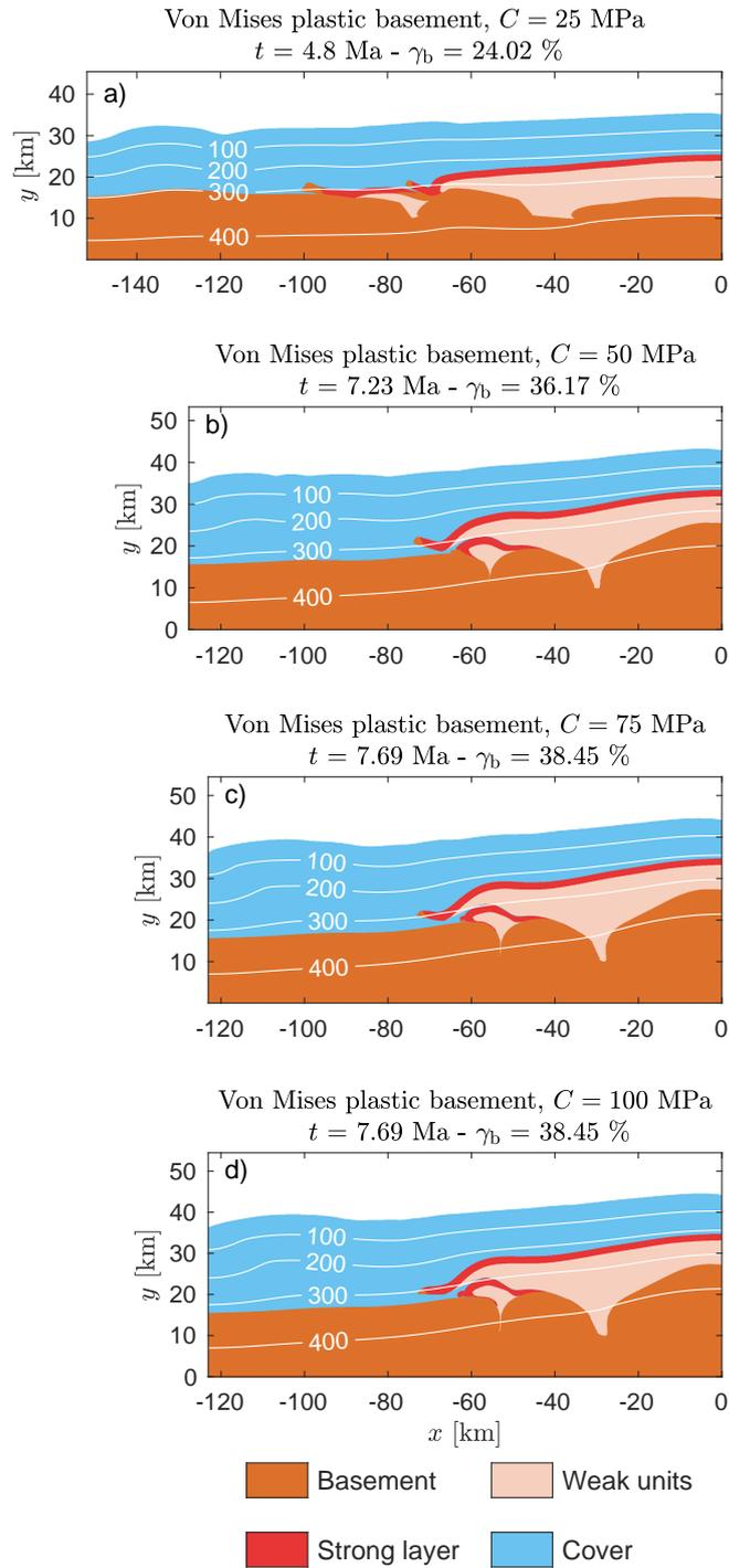
**Figure 8.** The final geometry and temperature fields of three simulations with different Von Mises yield criteria (see figure titles). The simulation with  $C = 25$  MPa has been terminated earlier, as the results (the sedimentary units are bulldozing off huge pieces of the crystalline basement) are totally different from geological observations.
