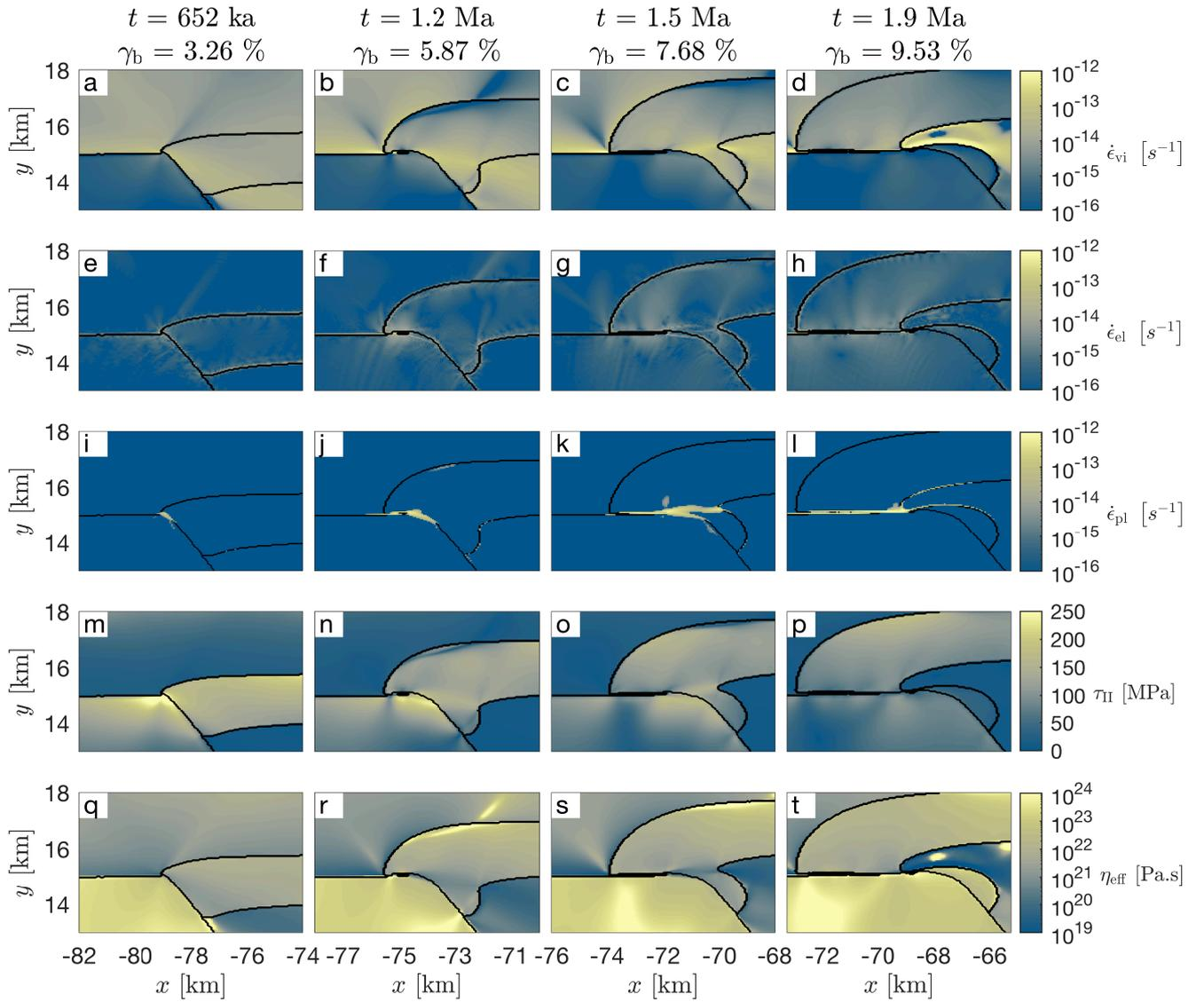
**Figure 5.** Enlargement of different stages of the detachment of the strong layer from the basement horst for different times,  $t$ , and bulk shortening,  $\gamma_b$  (see figure 4 for entire model domain). Colorplots of viscous strain rates (a-d), elastic strain rates (e-h), plastic strain rates (i-l), deviatoric stresses (m-p) and effective viscosities (q-t) are displayed. For all strain rate and stress tensor quantities we display their corresponding square root of the second invariants.
