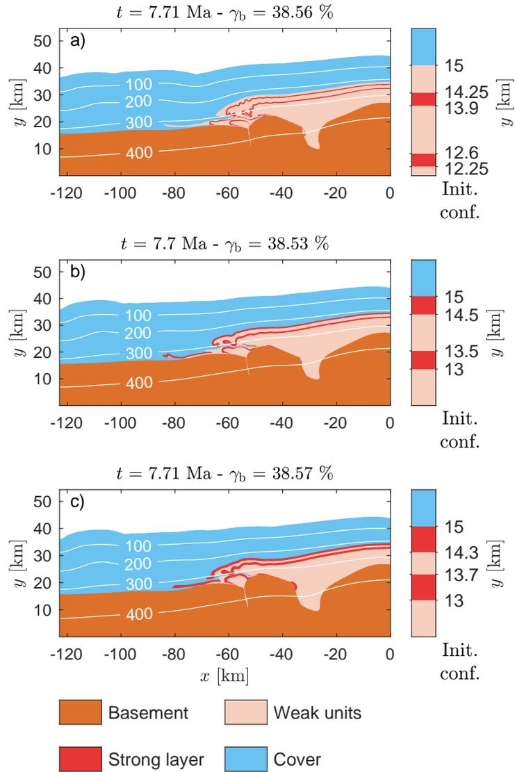
**Figure 9.** The final geometry of three simulations with two strong layers with the isotherms of the corresponding temperature field. The initial model stratigraphy around the upper region of the half-graben and basin is displayed on the right of each panel. The model stratigraphy is laterally homogenous, so the overall initial configuration is similar to that in Figure (2).
