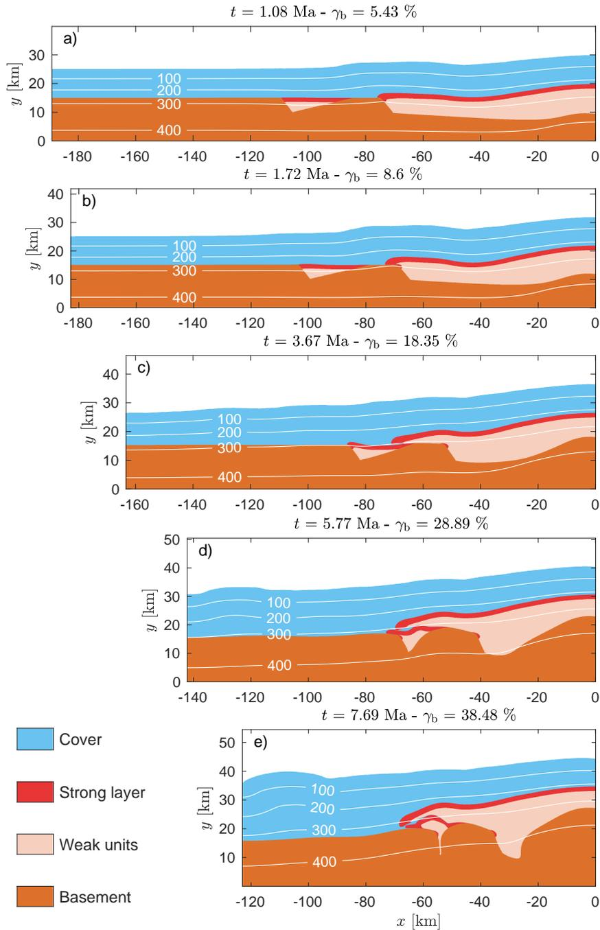
**Figure 3.** Structural and thermal evolution of the reference model for different times,  $t$ , and bulk shortening,  $\gamma_b$ . The white contours show isotherms and the labels are the corresponding temperatures in  $^{\circ}\text{C}$ . An animation, showing the full time evolution of the reference model, can be found as a supplementary material.
