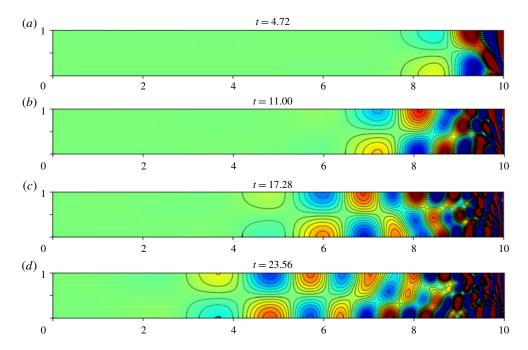
FIGURE 7. The analytic  $v^{wave}$ -contours in the  $E \downarrow 0$  limit at sequential times  $t = N\pi/2$ . (a) N = 3, (b) N = 7, (c) N = 11, cf. figures 3(c), (f), (i), respectively. (d) N = 15 (colour scale from -0.5 to 0.5).
