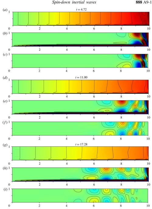
FIGURE 3. As in figure 1 but now v-contours for the same instants, at which  $E^{-1/2}\overline{v}_{MF}=0$ (equivalent to  $E^{-1/2} \overline{\chi}_{MF}$  maximised). Panels (a,d,g) show  $E^{-1/2} v_{DNS}$  (colour scale from -30 to 30); (b,e,h) and (c,f,i) show  $v_{FNS}$  and  $v_{IW}$ , respectively (colour scale from -0.5 to 0.5).
