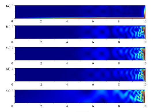
FIGURE 5. The meridional speed  $E^{-1/2}\sqrt{u^2 + w^2} = r^{-1}|\nabla(r\chi)|$  at t = 18.07 as in figure 2(g-i). Respectively, the panels show results for: (a-c) the filtered DNS  $\chi_{FNS}$ , when  $(a) E = 10^{-3}$ ,  $(b) E = 10^{-5}$ ,  $(c) E = 10^{-7}$ ; (d) the analytic  $\chi^{wave}$  in the limit  $E \downarrow 0$ ; (e) the full DNS  $E^{-1/2}\chi_{DNS}$  when  $E = 10^{-7}$  (colour scale from 0 to 3).
