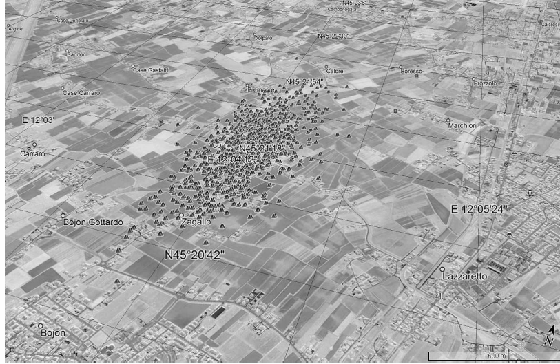
Fig. 15. A Google Earth maps showing the possible impact points on the ground obtained from the Monte Carlo simulation. The strewn field dimension is about 1.7 \times 0.6 km, about north of the town of Bojon.
