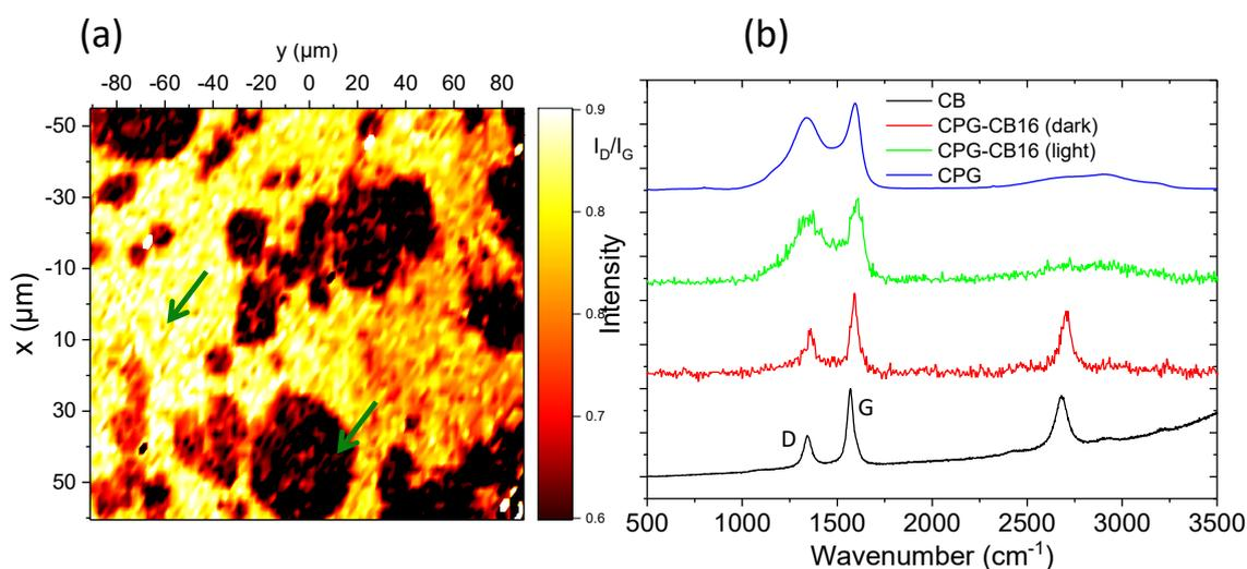
**Figure 2.** (a) Raman image reconstruction showing the  $I_D/I_G$  ratios for samples CPG-CB16; (b) Raman spectra of CB, CPG, and two different positions in the reconstructed Raman mapping for sample CPG-CB16 corresponding to dark and light areas (see arrows in plot a).
