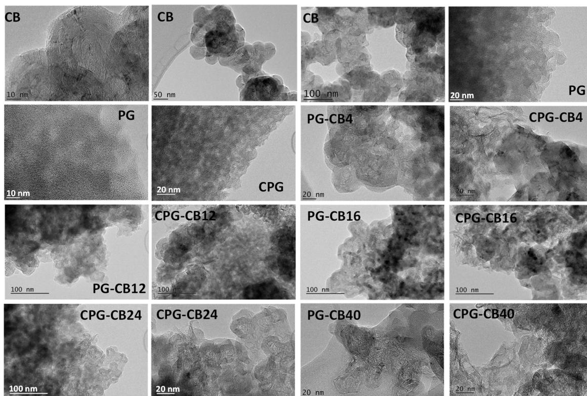
**Figure 1.** Selected TEM images of the carbon black additive, and the organic (series PG) and carbon gels (series CPG) prepared with different amounts of carbon black. For clarity, images are shown at various magnifications.
