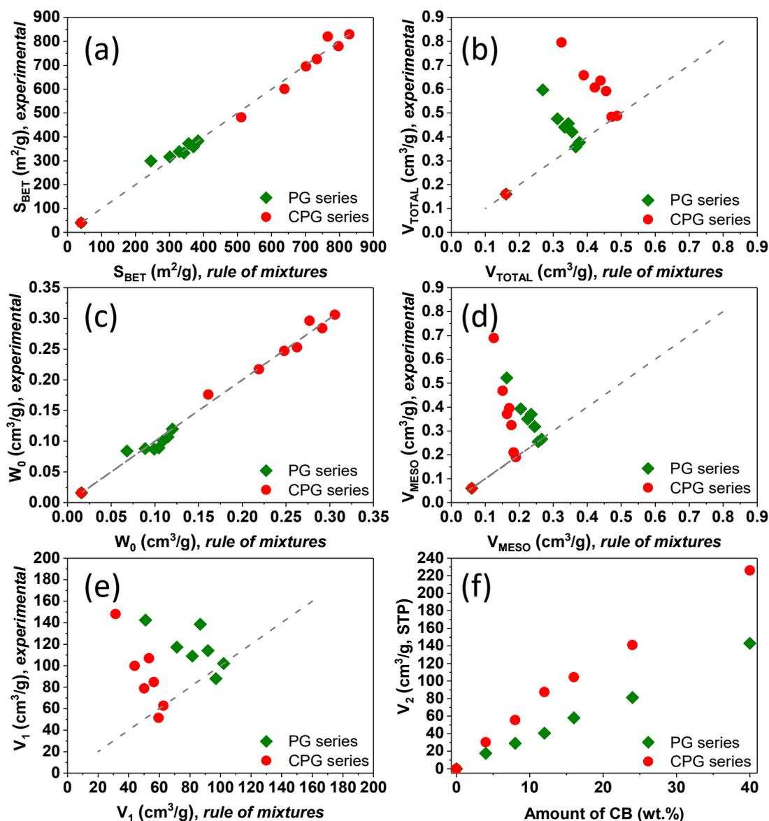
**Figure 4.** (a–e) Correlation of selected experimental textural parameters (surface area, pore volumes) of the gels/CB composites with the values predicted by the general mixing rule. Dashed lines indicate the expected trend following predictions of the general mixing rule. (f) Evolution of  $V_2$  with the amount of carbon additive.
