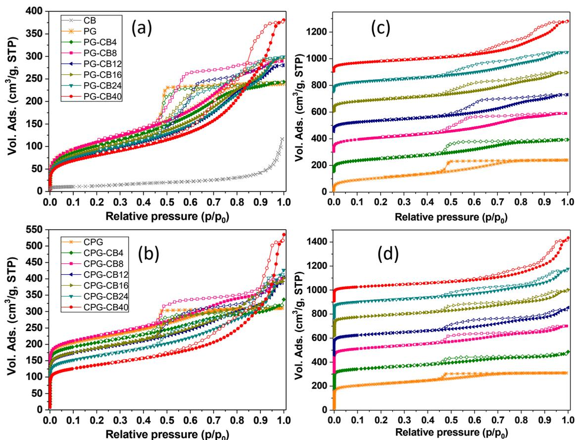
**Figure 3.** (a,b)  $N_2$  adsorption/desorption isotherms at  $-196^\circ\text{C}$  of the organic and carbon gels synthesized with different amounts of CB additive. Data corresponding to the carbon black are also shown as references. Isotherms in plots (c,d) have been shifted ca.  $150\text{ cm}^3/\text{g}$  for clarity.
