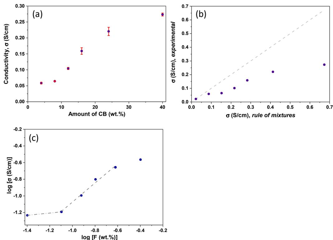
**Figure 6.** (a) Correlation of the electrical conductivity with the amount of carbon black; (b) correlation between the experimental conductivity and the values predicted by the general mixing rule; (c) log–log plot of the conductivity as a function of the amount of conductive phase following a percolation model.
