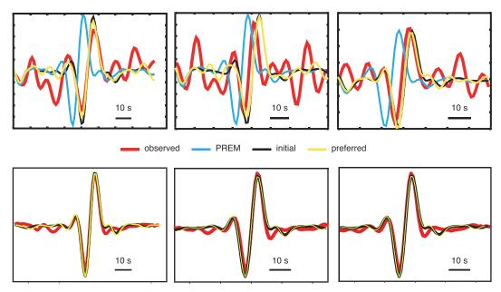
**Figure 9.** Upper panels: a comparison between observed waveforms, in red, and synthetic waveforms in blue, black, and yellow, computed via PREM, the initial model, and the preferred model, respectively. Lower panels: stacked waveforms of the seismic events from the upper panels.
