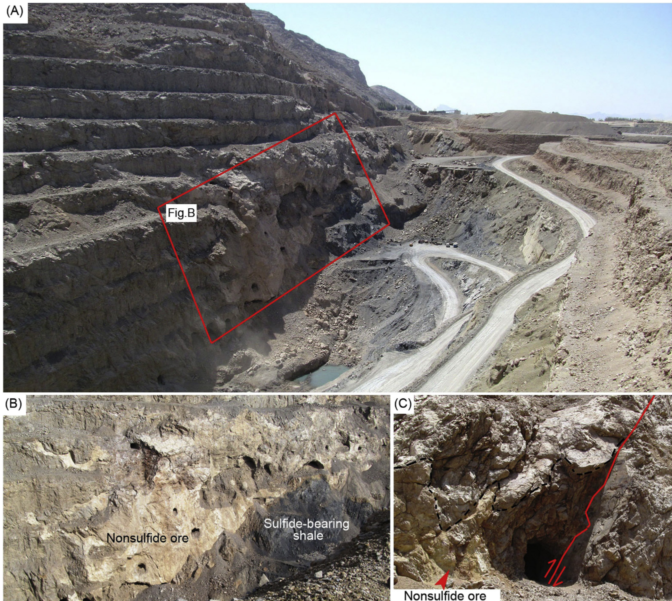
Figure 13. (A) Overview of the Kolahdarvazeh mine. The non-sulfide zinc ore occurs in the Early Cretaceous carbonate rocks. (B) Sphalerite, galena, and pyrite can be found within shales and adjacent to the non-sulfide zinc ore hosted by carbonate rocks. (C) View of the cavities and of the fault-breccias, originally filled by the non-sulfide ore.
