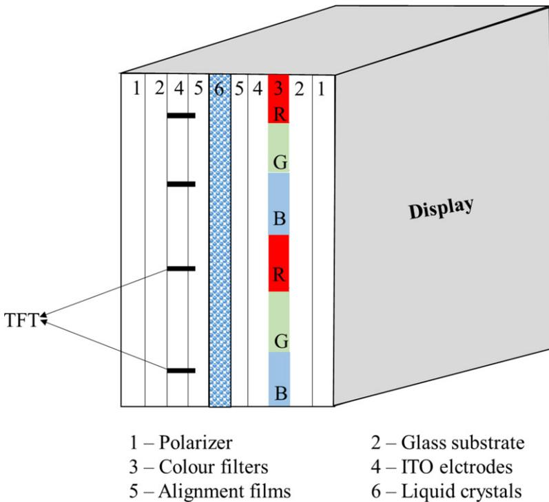
**Figure 4.** Cross section of a thin-film-transistor-LCD panel.
