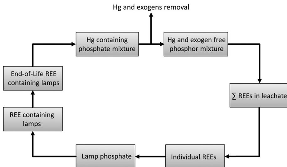
**Figure 11.** Recycling routes for SFLs (Binnemans et al., 2013).
