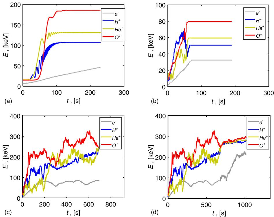
**FIG. 2.** Temporal changes of energies of the electron  $e^-$ , proton  $H^+$ , helium ion  $He^+$ , and oxygen ion  $O^+$  having the same initial positions and velocities during 4 different scenarios of magnetic perturbations: A [(a)], B [(b)], C [(c)], and D [(d)].
