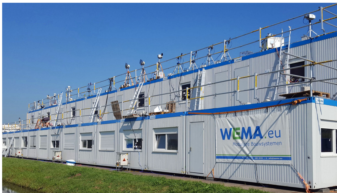
Figure 1. Picture of the CINDI-2 container layout at the main campaign site showing the organisation of the MAX-DOAS instruments on two superposed rows of mobile units (similar to shipping containers).
