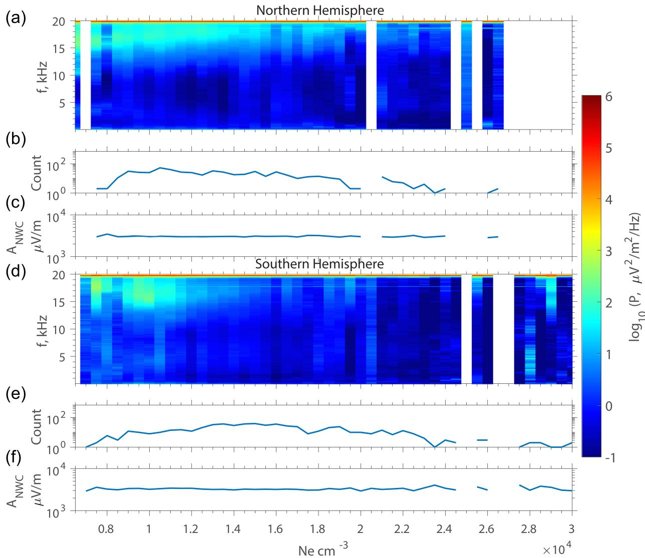
**Figure 4.** Panels (a) and (d) are the VLF electric wave power spectra versus frequency (y-axis) and plasma density (x-axis) at nightside in the northern and southern hemispheres, respectively. Panels (b) and (e) are the corresponding numbers of spectra in each density bins. Panels (c) and (f) are the corresponding mean NWC amplitude in each density bins.
