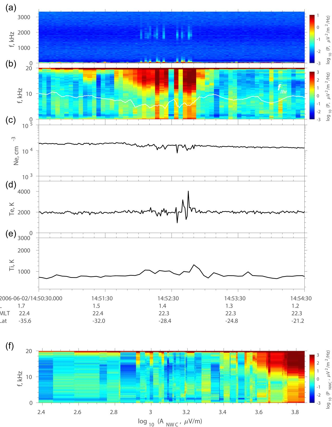
**Figure 1.** Overview of the spectral broadening event. (a) The electric wave power spectra in the HF band; (b) the electric wave power spectra in the VLF band; (c) the variation of electron density; (d) the variation of electron temperature; (e) the variation of ion temperature; (f) the VLF power spectra as a function of the amplitude of NWC signal. The white solid line in panel (b) denotes the lower hybrid resonance frequency.
