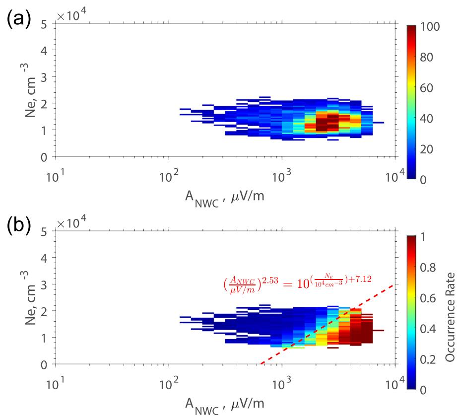
**Figure 5.** Panel (a) is the distribution of the number of occurrence with broadening spectra versus plasma density (y-axis) and NWC transmitter wave amplitude (x-axis). Panel (b) is the distribution of the spectral broadening occurrence rate.
