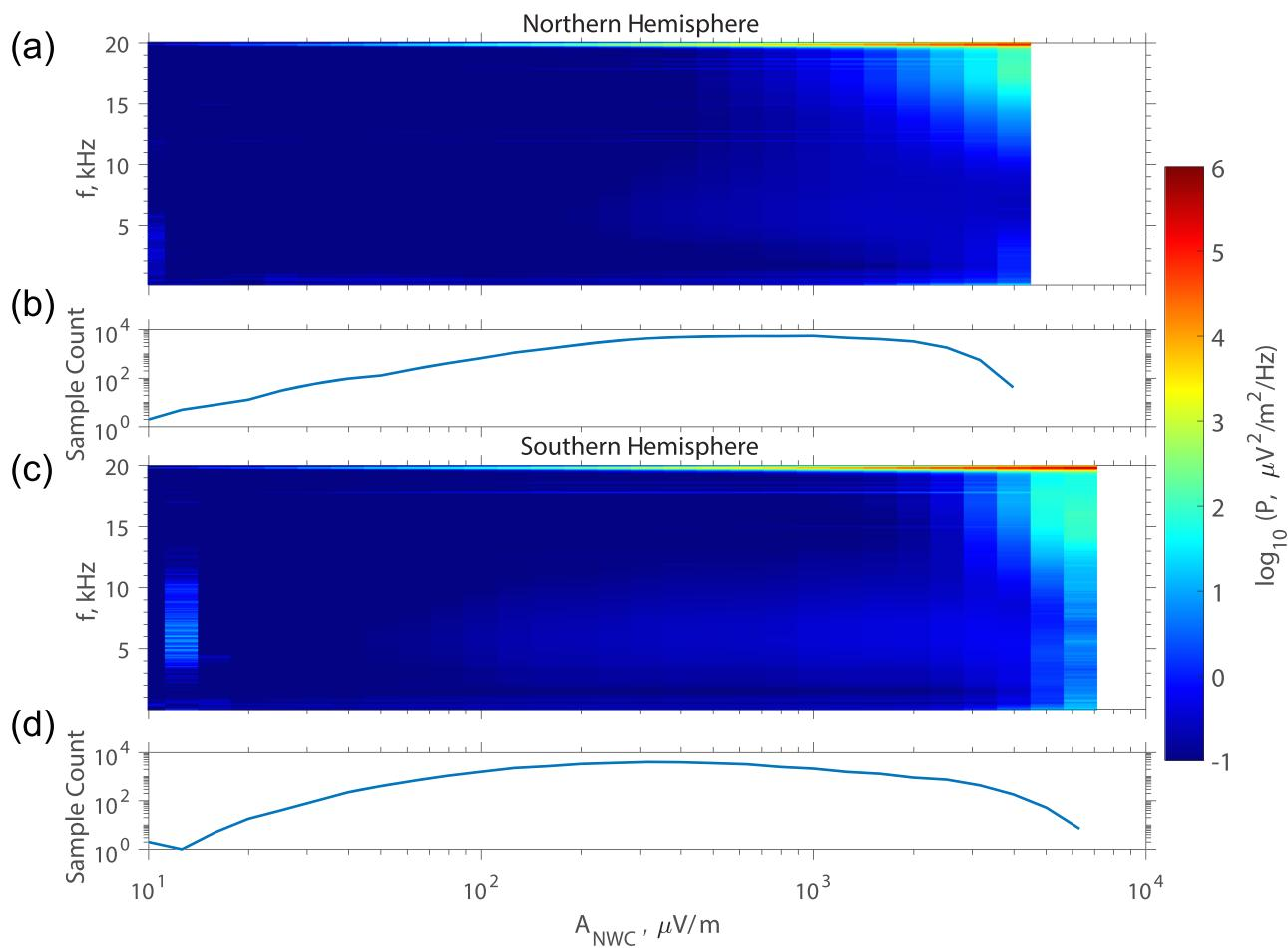
**Figure 3.** (a) and (c) are the VLF electric wave power spectra versus frequency (y-axis) and NWC amplitude (x-axis) at nightside in the northern and southern hemispheres, respectively. (b) and (d) are the corresponding numbers of spectra in each NWC amplitude bins.
