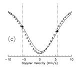
Figure 4: Schematic representation of the possible causes for the intensity changes observed in Figure 3. The triangles represent the absorption profile at rest. (a) blueshift: Upward motion to chromosphere. (b) redshift: Plasma is falling. (c) Reduced excitation of sodium: whole profile rises down, always with a redshift.
