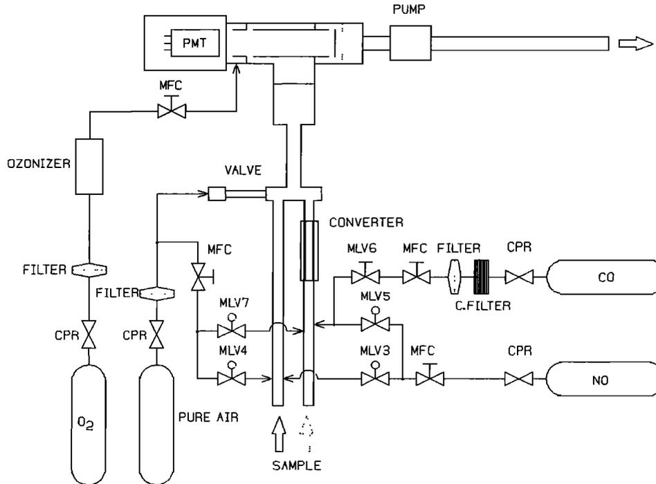
Fig. 1. Schematic diagram of the NO/NO<sub>2</sub> instrument used for the flight on June 18, 1988. MLV, magnetic latch valve; MFC, mass flow controller; CPR, constant pressure regulator; PMT, photomultiplier tube; and C. Filter, charcoal filter.
