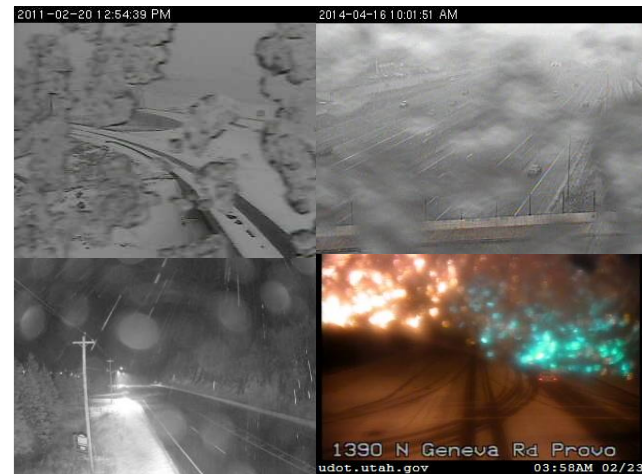
fig.5. Webcam images are often corrupted by natural masks (snowflakes, droplets, filth) and numerical overprints (text, logos, marks, etc).
