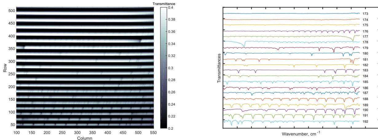
**Fig. 1.** *Left panel:* example of a single detector frame measured by ACS MIR in secondary grating position 12 after processing (orbit 6975,  $L_s = 40.3^\circ$ , tangent altitude 13 km). *Right panel:* associated series of transmission spectra, covering the wavenumber range from  $2894 \text{ cm}^{-1}$  (diffraction order 173) to  $3239 \text{ cm}^{-1}$  (order 192). The left and right edges of the frame in the spectral dimension, where the signal decreases, are cropped.
