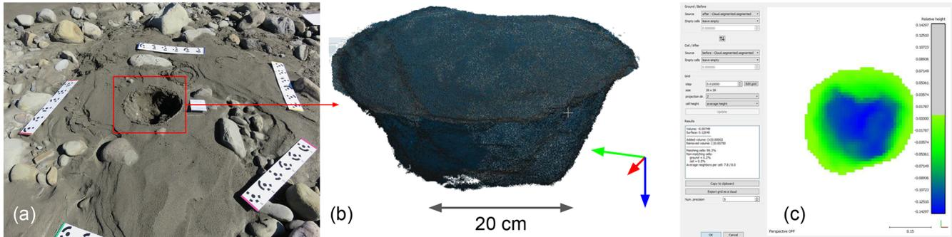
**Figure C1.** (a) Picture of the hole taken with references scales and benchmarks. Several pictures were thus taken before and after the hole was dug. (b) 3-D cloud of the points mapping the surface of the hole. (c) Computation of the volume bounded by the hole and the former surface of the ground before the hole was done.
