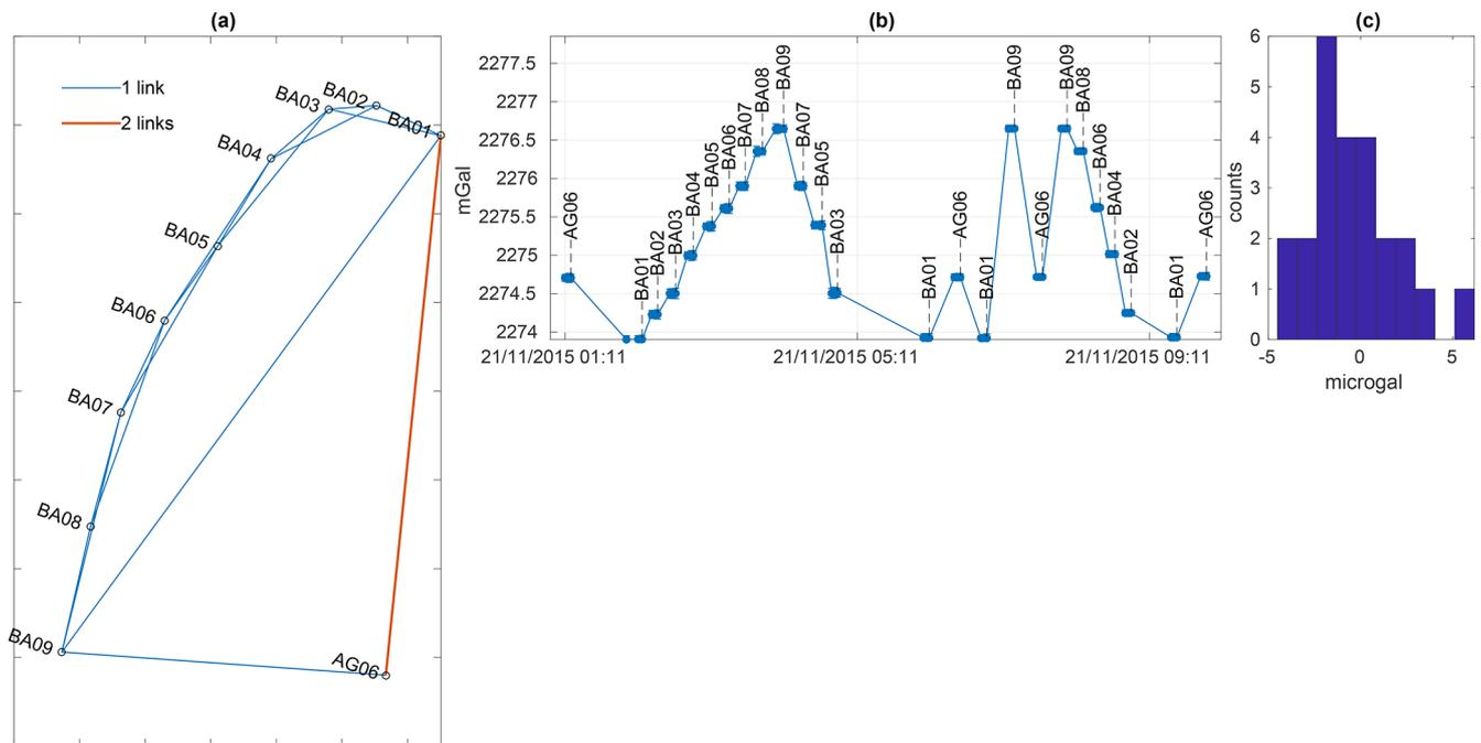
**Figure A1.** (a) Map view of the relative gravity network with the link between each site for the 2015 survey. (b) Gravity readings on the CG-5 at each site as a function of time. (c) Histogram of the residuals after the drift adjustment.
