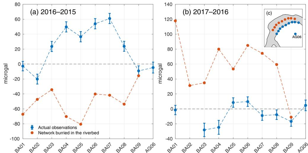
**Figure 11.** Gravity changes expected at new sites located 5 m beneath the river (red), compared with those measured at BA01–BA09 (blue), for the same sediment mass redistributions as (a) between 2015 and 2016 and (b) between 2016 and 2017. The new sites are in fact BA01–BA09 translated 140 m in the northeast direction, as illustrated in (c).
