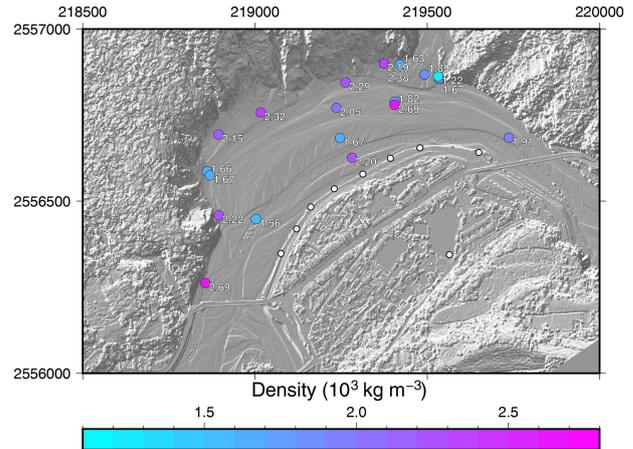
**Figure 8.** In situ density measured during the 2017 survey (colored dots; the value is also reported in white). Gravity sites are shown with white dots. Axes are in meters. The background is the shaded topography measured during the 2017 survey.
