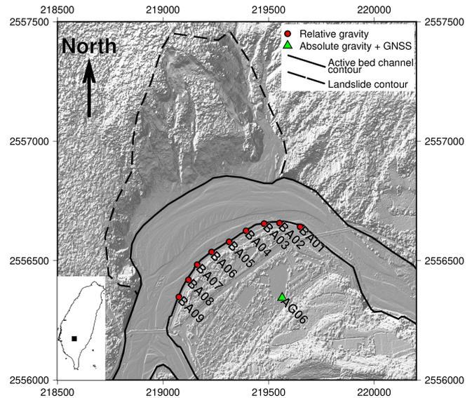
**Figure 1.** Shaded relief map of the study area. Absolute gravity measurements are performed only at AG06 while relative gravity measurements are performed at every site. The background image is the hill-shaded topography at half-meter resolution obtained by photogrammetry using an unmanned aerial vehicle (UAV). Map to the bottom left shows the study area in Taiwan. Axes are in meters in the TWD97 coordinate reference system.
