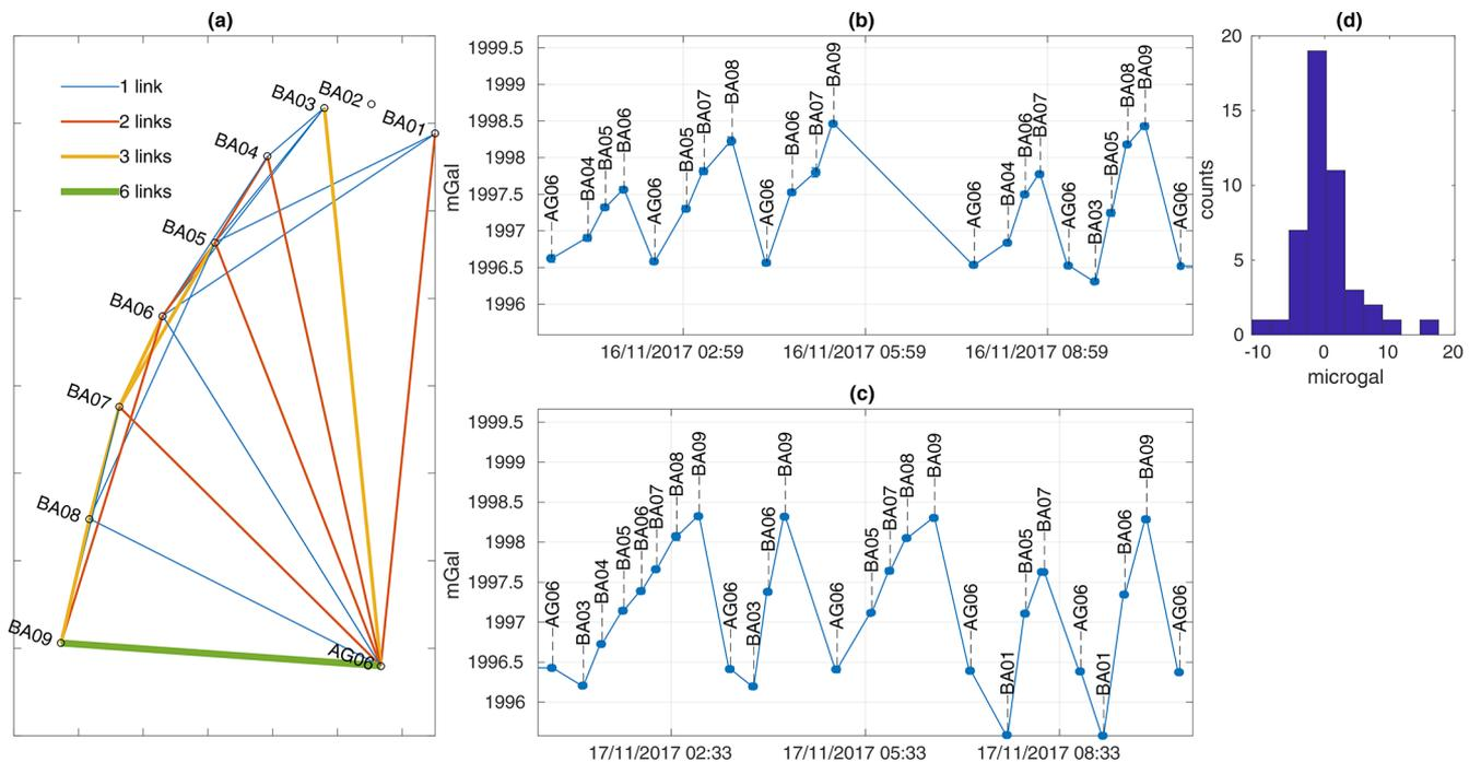
**Figure A3.** (a) Map view of the relative gravity network with the link between each site for the 2017 survey. (b, c) Gravity readings on the CG-5 at each site as a function of time. (d) Histogram of the residuals after the drift adjustment.
