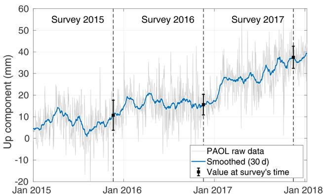
**Figure 4.** Ground vertical displacement time series at the PAOL GNSS station, collocated with AG06, provided by the GPLSLAB database (IES-AS, 2015). Solutions are computed in the IGS08 reference frame (Rebischung et al., 2012). The time of each joint gravimetry–photogrammetry survey is shown by dotted lines. The error bar is computed from the SD of the measurements of the same 30 d window.
