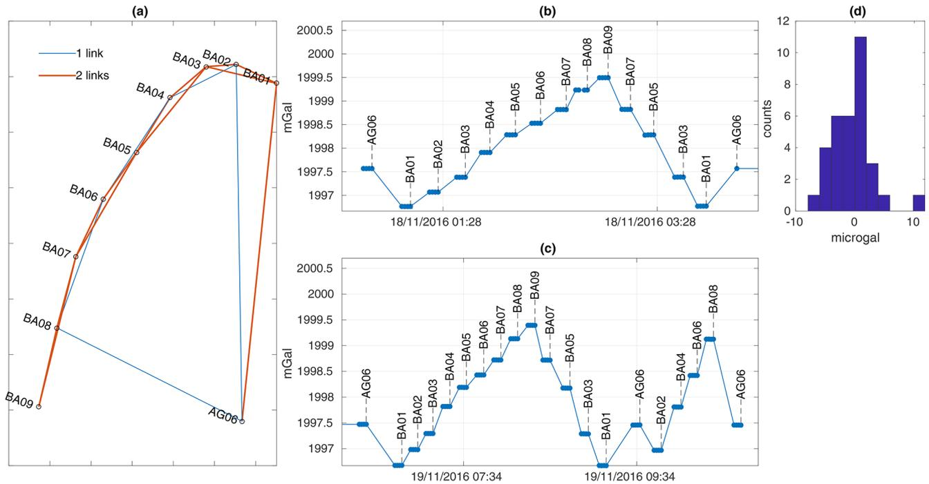
**Figure A2.** (a) Map view of the relative gravity network with the link between each site for the 2016 survey. (b, c) Gravity readings on the CG-5 at each site as a function of time. (d) Histogram of the residuals after the drift adjustment.
