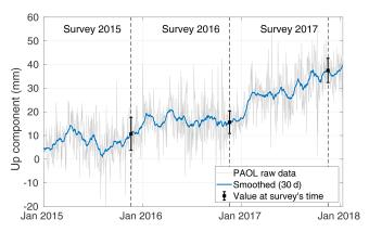
**Figure 4.** Ground vertical displacement time series at the PAOL GNSS station, colocated with AG06, provided by the GPSLAB database (IES-AS, 2015). Solutions are computed in the IGS08 reference frame (Rebischung et al., 2012). The time of each joint gravimetry–photogrammetry survey is shown by dotted lines. The error bar is computed from the SD of the measurements of the same 30 d window.
