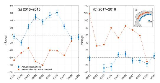
**Figure 11.** Gravity changes expected at new sites located 5 m beneath the river (red), compared with those measured at BA01–BA09 (blue), for the same sediment mass redistributions as (a) between 2015 and 2016 and (b) between 2016 and 2017. The new sites are in fact BA01–BA09 translated 140 m in the northeast direction, as illustrated in (c).
