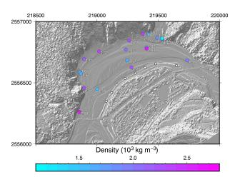
**Figure 8.** In situ density measured during the 2017 survey (colored dots; the value is also reported in white). Gravity sites are shown with white dots. Axes are in meters. The background is the shaded topography measured during the 2017 survey.
