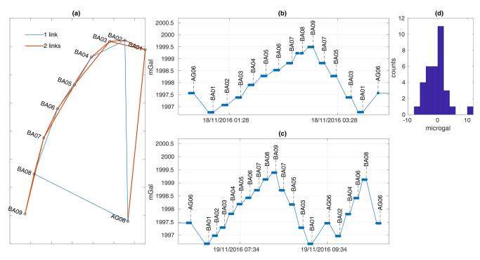
**Figure A2.** (a) Map view of the relative gravity network with the link between each site for the 2016 survey. (b, c) Gravity readings on the CG-5 at each site as a function of time. (d) Histogram of the residuals after the drift adjustment.
