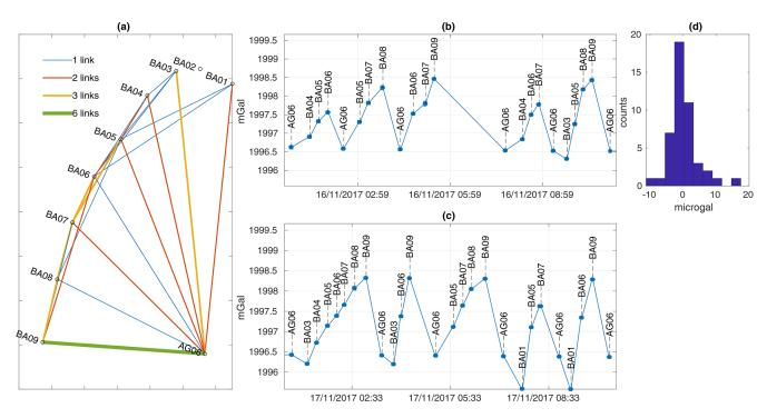
Figure A3. (a) Map view of the relative gravity network with the link between each site for the 2017 survey. (b, c) Gravity readings on the CG-5 at each site as a function of time. (d) Histogram of the residuals after the drift adjustment.
