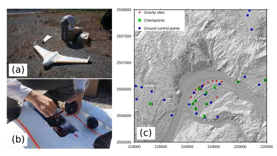
Figure 6. (a) Modified Skywalker X8 UAV. (b) Close-up on the central compartment of the UAV, where the camera and lens are mounted. (c) Map of the ground control points and checkpoints (numbered according to Table 4) with the shaded topography in the background. The gravity sites are also shown for reference.
