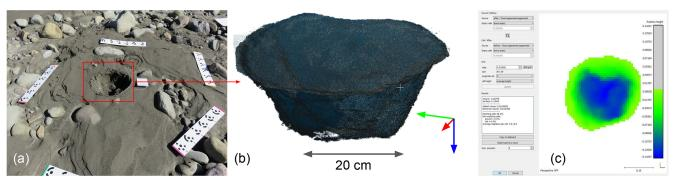
Figure C1. (a) Picture of the hole taken with references scales and benchmarks. Several pictures were thus taken before and after the hole was dug. (b) 3-D cloud of the points mapping the surface of the hole. (c) Computation of the volume bounded by the hole and the former surface of the ground before the hole was done.
