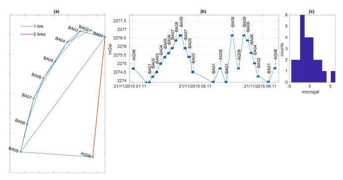
**Figure A1. (a)** Map view of the relative gravity network with the link between each site for the 2015 survey. **(b)** Gravity readings on the CG-5 at each site as a function of time. **(c)** Histogram of the residuals after the drift adjustment.
