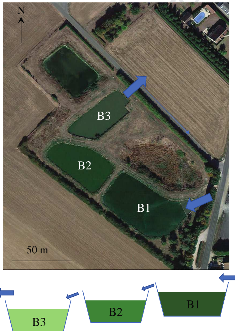
Figure 1: Lagoon-based system (with a schematic representation of its functioning) as wastewater treatment plant of the town of Josnes located in the Region Centre in France.
