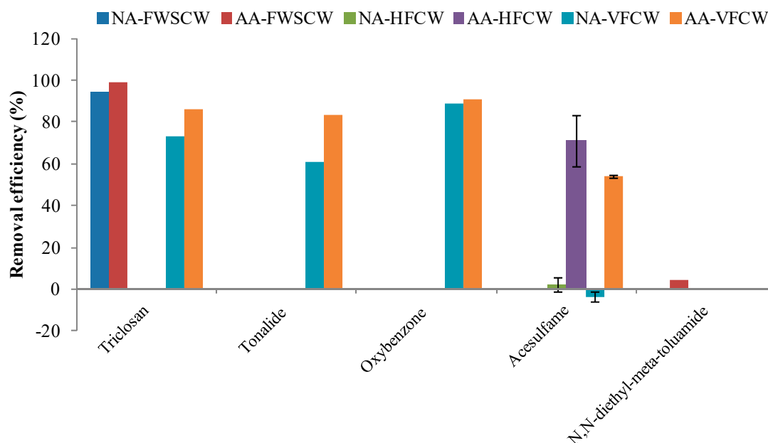
Figure 5. Removal efficiency of PCPs in different types of aerated (AA) and non-aerated (NA) CWs. Note: Data is taken from: Ávila et al. [22]; Li et al. [21]; Kahl et al. [17]; and Nivala et al. [18]. The enhanced removal is explicit in the case of AA-FWSCW (triclosan), AA-HFCW (acesulfame), AA-VFCW (triclosan, tonalide, oxybenzone, and acesulfame) compared with their corresponding NA-CWs.
