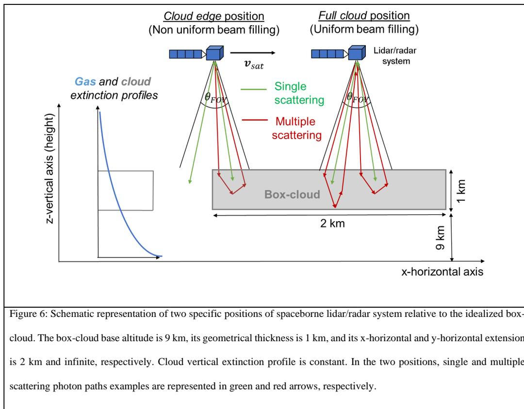
The box-cloud base altitude is 9 km, its geometrical thickness is 1 km, and its x-horizontal and y-horizontal extension is 2 km and infinite, respectively. Temperature and pressure vertical profiles assume 1976 U.S. standard atmosphere models. Optical
