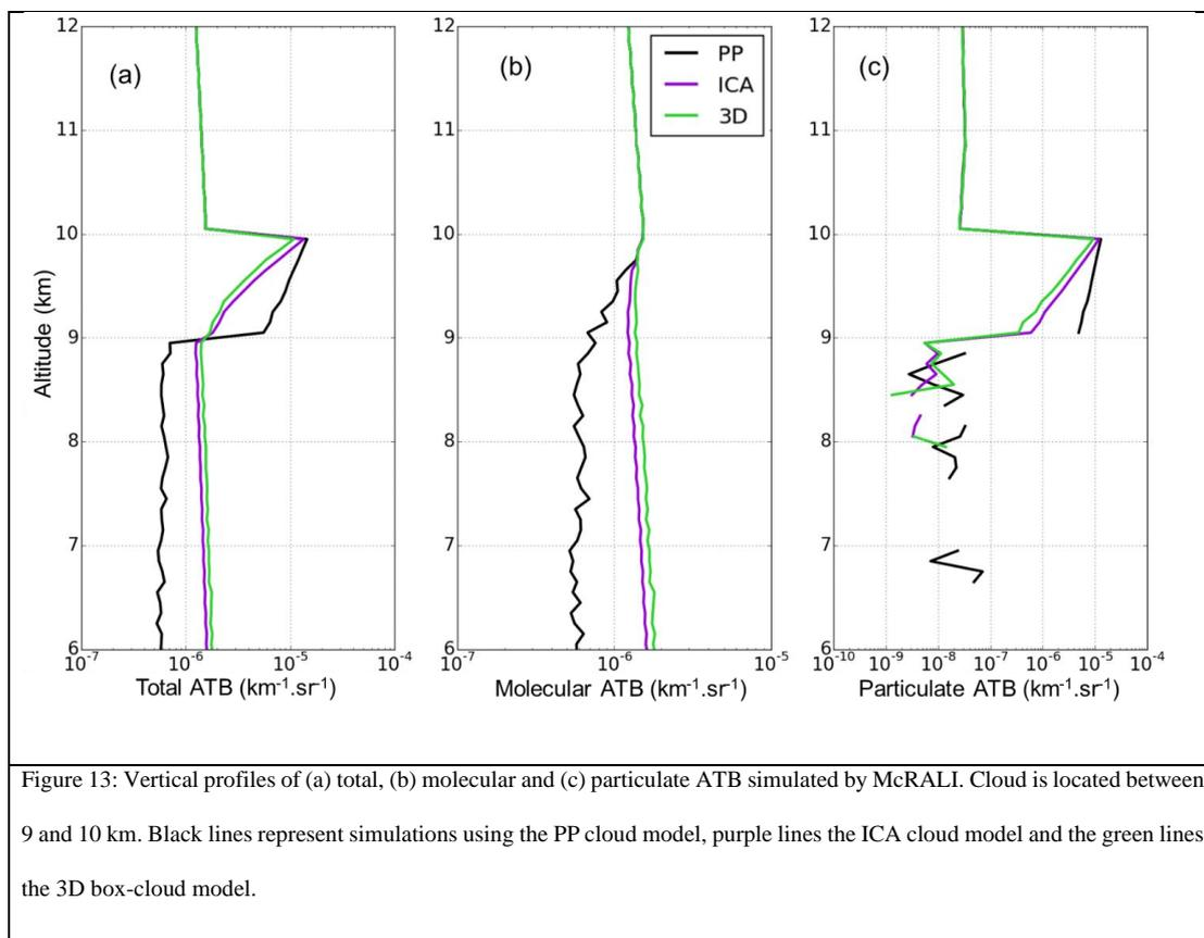
Figure 13: Vertical profiles of (a) total, (b) molecular and (c) particulate ATB simulated by McRALI. Cloud is located between 9 and 10 km. Black lines represent simulations using the PP cloud model, purple lines the ICA cloud model and the green lines the 3D box-cloud model.
