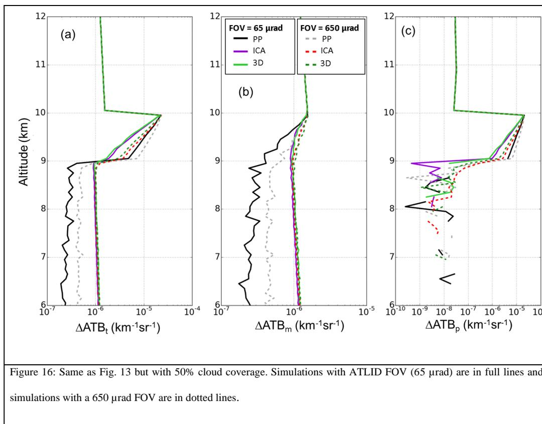
When comparing ATB computed with the three cloud models (i.e. PP, ICA and 3D cloud model) for the large FOV, the same conclusions as for the ATLID FOV can be made: when reaching the cloud base, total and particulate ATBs show lower values for ICA and 3D models than for PP model, and the opposite for the molecular ATB. Biases also show the same trend as for
