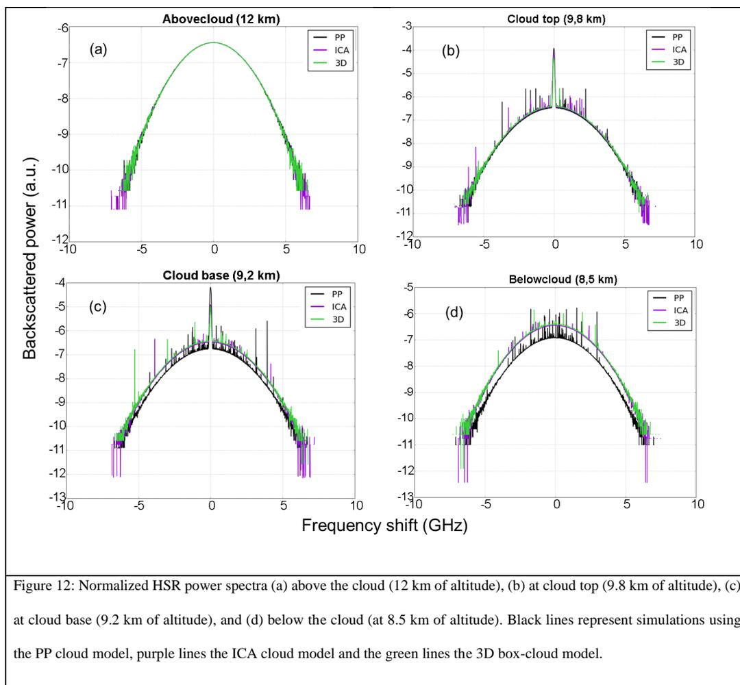
One can clearly see that the intensity of the central Mie (particulate) peak computed by ICA and 3D is lower than the one computed by the PP simulation. The opposite behaviour is observed concerning the Rayleigh (molecular) scattering region: the broad and low intensity spectra for ICA and 3D simulations show larger values (in intensity) compared to PP simulation, and for the full range of frequency shift. The same observation can be made below the cloud.
