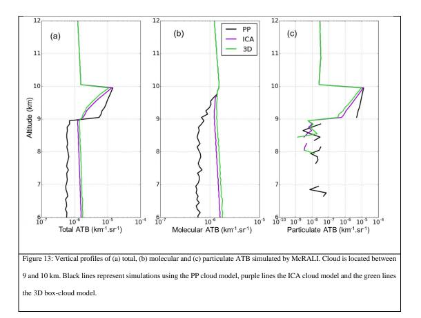
In order to obtain the molecular and particulate ATB vertical profiles for the three cloud models (Fig. 13b and Fig. 13c), the HSR spectra are filtered by a modelled Fabry-Perot interferometer (see Sect. 2.5.3 for the filtering parameters) at each altitude level. The ATB vertical profiles (Fig. 13a) exhibit features observed on HSR spectra more clearly: once the cloud is reached
