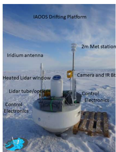
Fig. 1: Implementation of the instrumentation on the IAOOS platform
