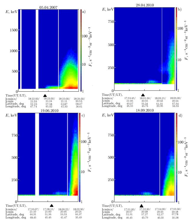
Fig. 2. Examples of the sessions in which the precipitations that could certainly be qualified as artificial (sessions 7, 15, 18, and 20 on panels *a*, *b*, *c*, and *d*, respectively) were not detected during the Sura operation.
