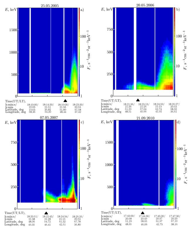
Fig. 4. Examples of the sessions where artificial precipitations were detected in the absence of ducts with increased plasma density (sessions 2, 5, 8, and 21 on panels *a*, *b*, *c*, and *d*, respectively).
