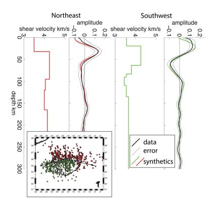
**Figure 5.** Waveform modeling of Sp data from the simultaneous deconvolution. Sp data (black) binned by conversion point bins at 100 km depth into 2 bins (red and green dots in inset map) are compared to synthetics from forward modeling for the southwest (green) and northeast (red). Corresponding shear velocity profiles are shown to the left of the data/ synthetics plots. Error bars indicating 95% confidence from bootstrap are shown in grey.
