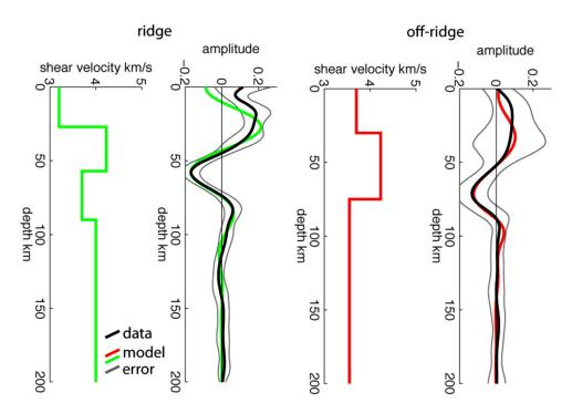
**Figure 4.** Waveform modeling of Sp 3-D multitaper model (black) beneath the ridge and beneath the 9 My age contour (locations of triangles in Figure 3) are compared to synthetics from forward modeling (red and green lines). Corresponding shear velocity profiles are shown to the left of the data/synthetics plots. Error bars indicating 95% confidence from bootstrap are shown in grey.
