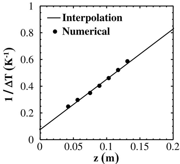
**Figure C4.** Axial temperature anomaly as a function of height  $z$  for one numerical simulation. The solid line corresponds to proportionality constant  $C_n = 0.49$ , close to the theoretical value for large Prandtl numbers.
