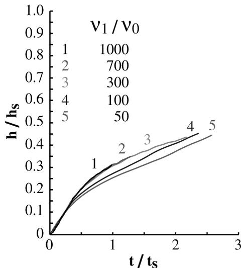
**Figure 18.** Dimensionless interface position as a function of dimensionless time  $t/t_s$  for five calculations at different values of viscosity ratio  $\nu_1/\nu_0$  with all other parameters kept constant ( $B = 0.78$ ).
