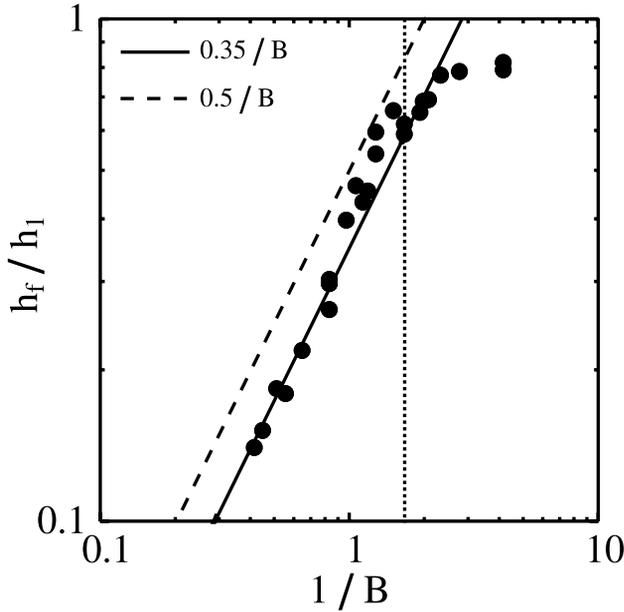
**Figure 16.** Dimensionless interface position  $h_f/h_1$  at the end of the first deformation phase, before the onset of convection in the upper fluid, as a function of  $1/B$ . The dashed line corresponds to the fully developed linear temperature profile shown on Figure 15. The solid line corresponds to a best fit through the data points. The vertical dotted line corresponds to  $B = 0.6$ , which separates the two different plume regimes.
