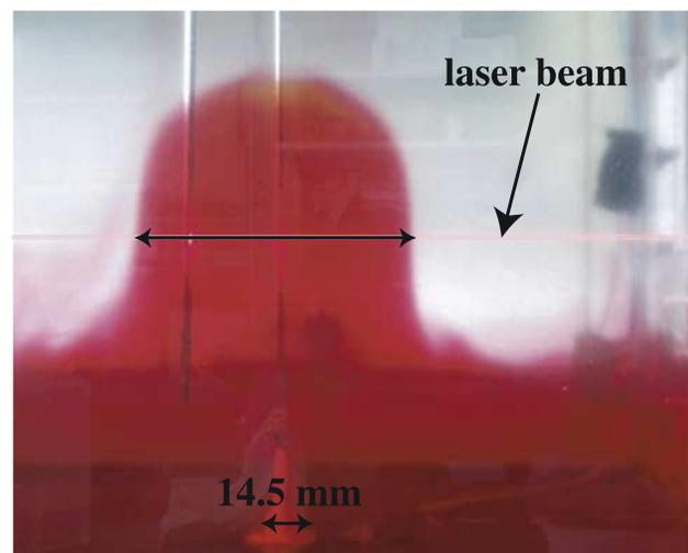
**Figure A1.** A well-deformed interface in experiment 17 with a horizontal laser beam which is used to determine the top of the interface and the width of the deformed region. The small heater used to generate a thermal plume in the lower liquid is seen at the bottom.
