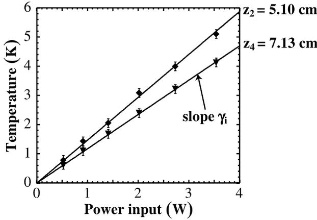
**Figure C1.** Axial temperature anomaly in experimental plumes as a function of power input for two different heights above source. Plume temperature is proportional to power input, as predicted by theory. Slope  $\gamma$  is used to determine the location of the virtual point source for the plume.
