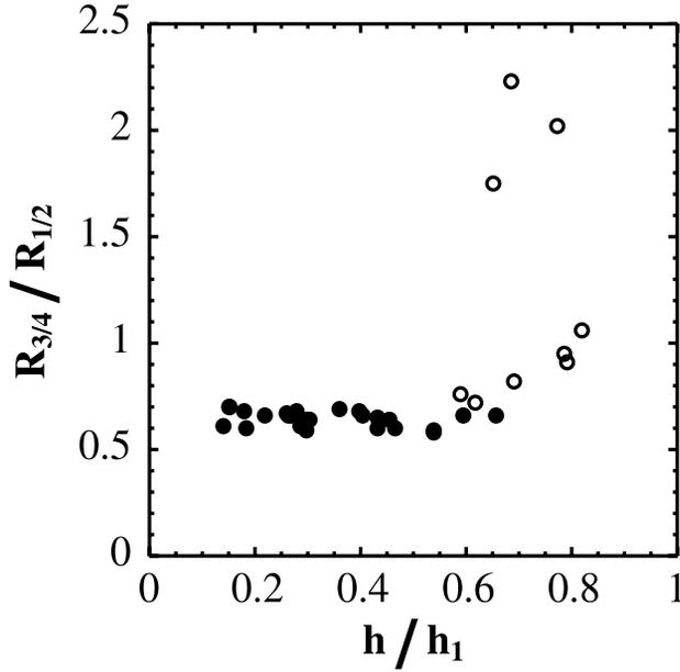
**Figure 12.** Shape ratio for the deformed interface,  $R_{3/4}/R_{1/2}$ , as a function of dimensionless interface height  $h/h_1$ . Solid symbols are  $B > 0.6$ . Open symbols are  $B < 0.6$ . In the interface deformation mode ( $B > 0.6$ ),  $h/h_1$  is less than 0.6, and the interface is deformed into a Gaussian bell. In the plume penetration mode ( $B < 0.6$ ),  $h/h_1$  takes larger values which typify the tall intrusion that develops.
