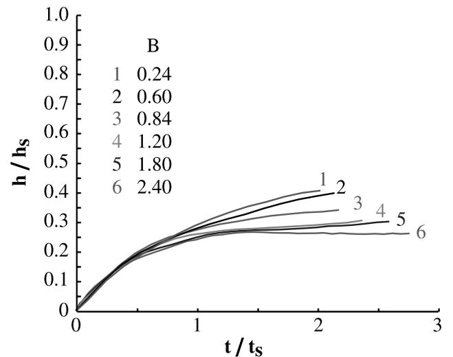
**Figure 17.** Dimensionless interface position  $h/h_s$  as a function of dimensionless time  $t/t_s$  for six calculations at different values of  $B$  with all other parameters kept constant ( $\nu_1/\nu_0 = 100$ ).
