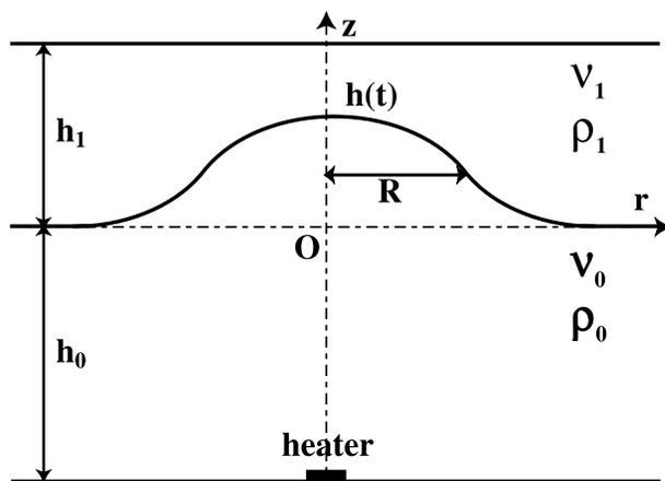
**Figure 1.** Model system of two layers with a basal heat source to generate a thermal plume. The plume induces deformation of the interface between the two layers;  $h(t)$  denotes the maximum interface displacement at the axis.
