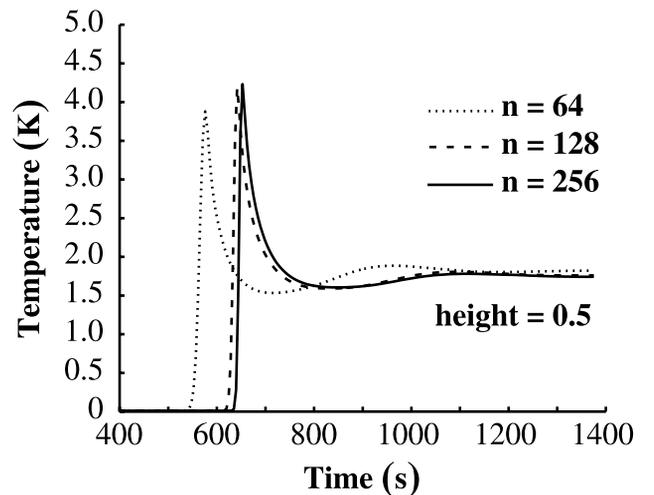
**Figure C3.** Axial temperature anomaly from numerical simulations as a function of time for three different grid sizes. Note that the largest grid size ( $n = 64$ ) allows poor time resolution but good prediction of temperature values.
