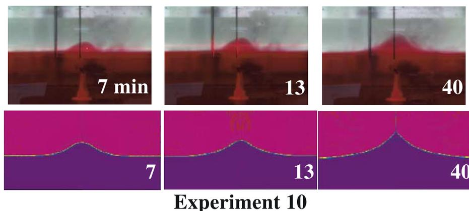
**Figure 7.** (top) Experiment 10 at  $B \approx 1.2$  and  $\nu_1/\nu_0 = 18$ . (bottom) Numerical analogue (simulation 36). Plots are drawn on the same scale, allowing direct comparison between the two. One may see that the numerical calculation reproduces the dimensions of the intrusion quite well. At  $t = 40$  min, the upper layer has developed an active convective upwelling, and the intrusion has been distorted into a cusp. The numerical calculation has a slightly sharper cusp.
