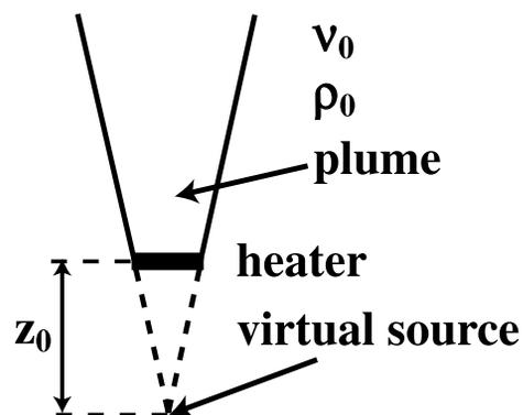
**Figure 2.** Schematic diagram showing how a plume generated by heating over a finite lateral distance can be referred to a virtual point source located below the heater. Laboratory experiments and numerical calculations are set up so that they have the same virtual point source and power input.
