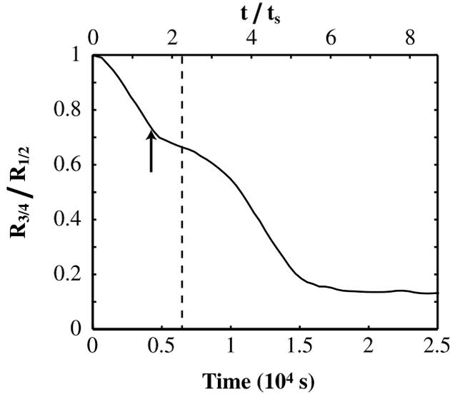
**Figure 10.** Shape ratio  $R_{3/4}/R_{1/2}$  versus time for simulation 19 ( $B = 1.2$ ). The shape ratio is approximately 0.6 for a Gaussian bell-shaped intrusion and drops to values less than 0.5 for a cusp. The dashed line separates the two different phases of interface deformation at the inflection point. The onset of convection in the upper layer occurs earlier at the time indicated by the arrow.
