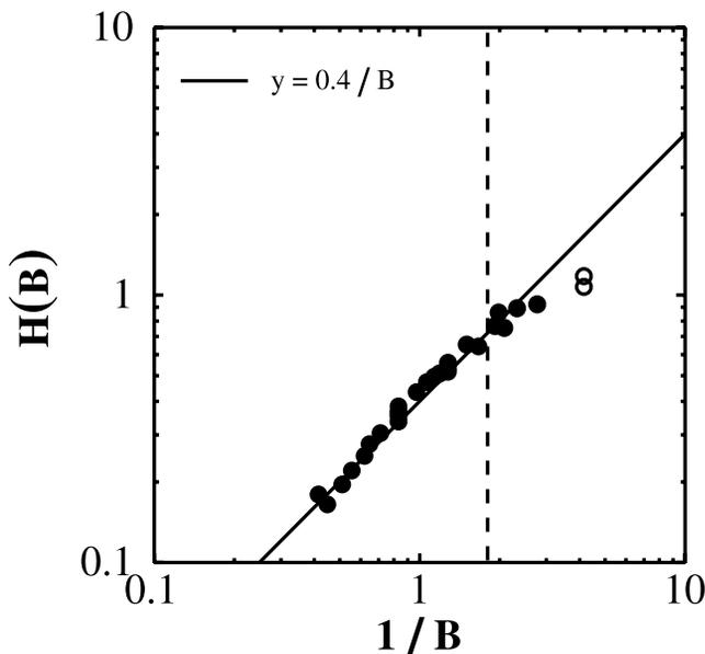
**Figure 14.** Dimensionless function  $\mathcal{H}(B)$  for the initial rate of vertical deformation, as a function of  $B$  for all numerical calculations. Open symbols correspond to calculations 23 and 30 at very low values of  $B$ , such that plume penetration is very rapid and proceeds almost to the top of the upper layer. The vertical dashed line corresponds to  $B = 0.6$ , which separates the two different plume behaviors.
