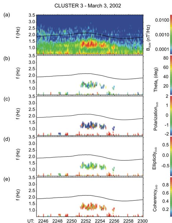
**FIGURE 4:** (a) Magnetic field spectral measurements in the frequency range 0.5 to 3.5 Hz showing the presence of Pc1 waves around 1.2 – 1.7 Hz from 22:51 to 22:55 UT. (b) Theta angle of the  $\mathbf{k}$  vector; (c) Polarization of the waves; (d) Ellipticity of the waves; and (e) coherency of the waves, using the SVD method as applied to the data plotted in panel (a)
