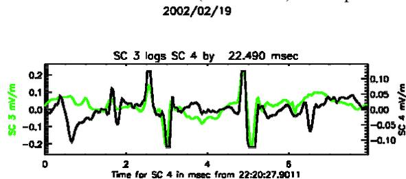
**FIGURE 1.** Example of ESW propagation from Cluster SC4 to SC3 where the SC3 waveforms have been brought forward in time by the detected lag to SC4 (22.49 ms) and overlaid on the SC4 waveforms. (Extracted from Figure 5 of Pickett et al., [16])
