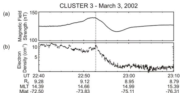
**FIGURE 2.** Magnetic field strength and density measurements on Cluster 3 while the spacecraft is in the magnetopause boundary layer on the earthward side. The dashed line indicates the time at which the data plotted in Figure 3 were obtained.
