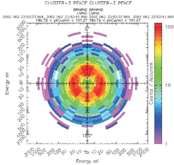
**FIGURE 5.** Cross section of the electron energy distribution function during the ESW measurements shown in Figure 3(a). Electron beams of a few tens of eV are present at parallel and antiparallel to the local magnetic field, as well as at 45 degrees to magnetic field direction.
