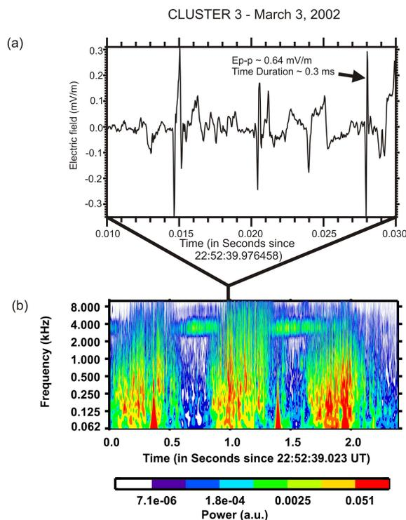
**FIGURE 3.** (a) Example of ESWs detected on Cluster 3. (b) Wavelet spectrogram showing bursts of electrostatic waves in the frequency range 0.1 - 4 kHz and narrow-banded waves (probably whistler mode) around 3.5 - 4.0 kHz. The electrostatic bursts are comprised of ESWs as shown by the location of the waveform sample in Figure 3(a).
